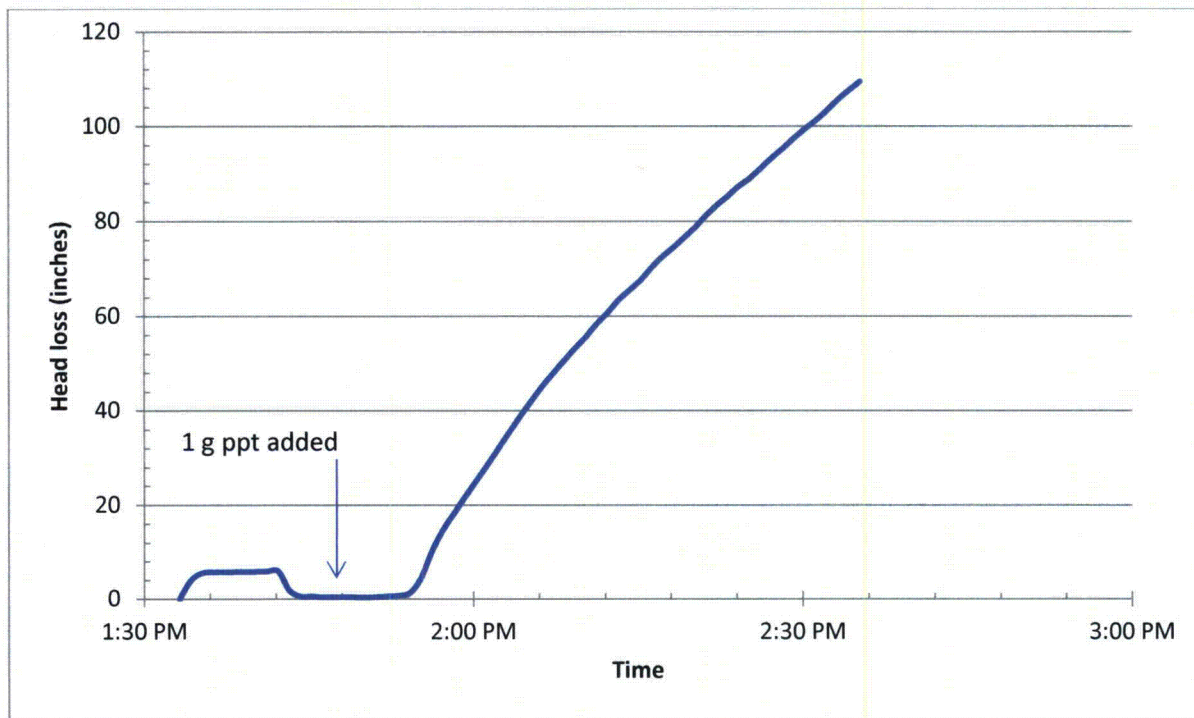
Figure 18: Head loss in Test 12 with fiber bed prepared with a blender and addition of WCAP precipitate.
