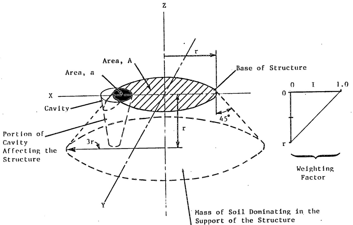
Fig. E-1 DIAGRAM DESCRIBING THE EFFECT OF THE CAVITY ON THE STRUCTURE
