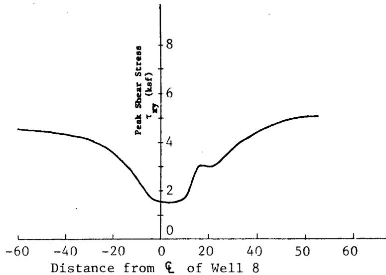
Fig. C-5 DISTRIBUTION OF PEAK SHEER STRESS THROUGH TYPICAL SECTIONS DUE TO DBE
