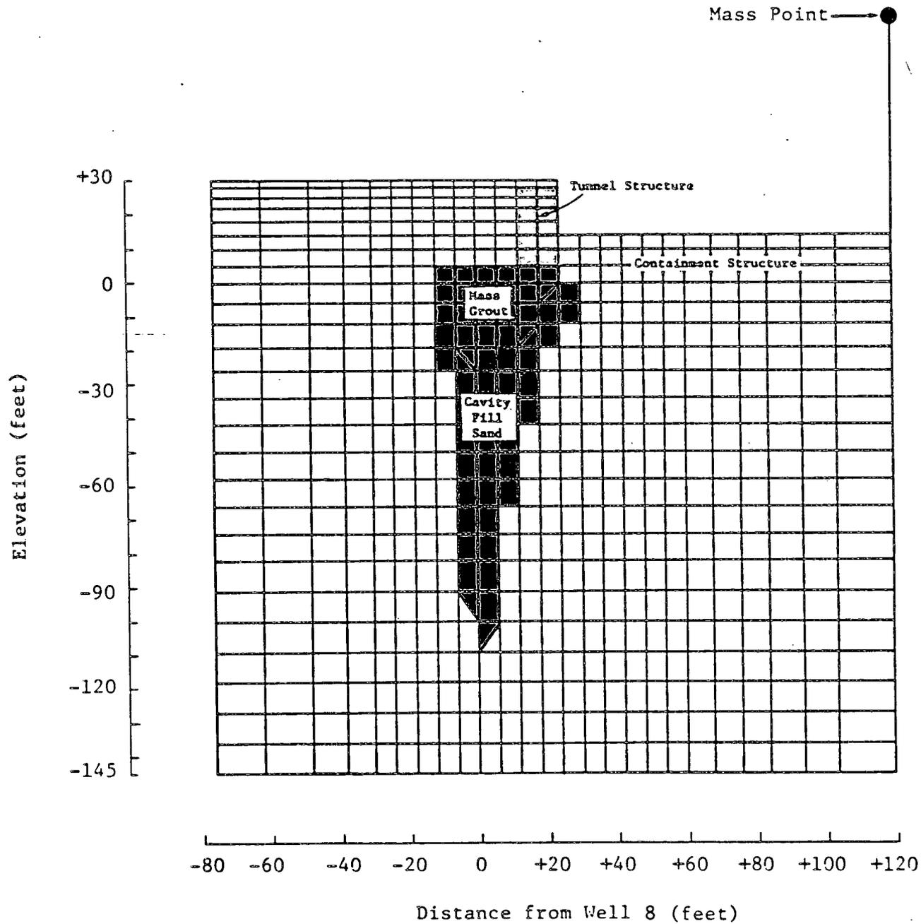
Fig. 5 FINITE ELEMENT MESH USED IN ANALYSIS
