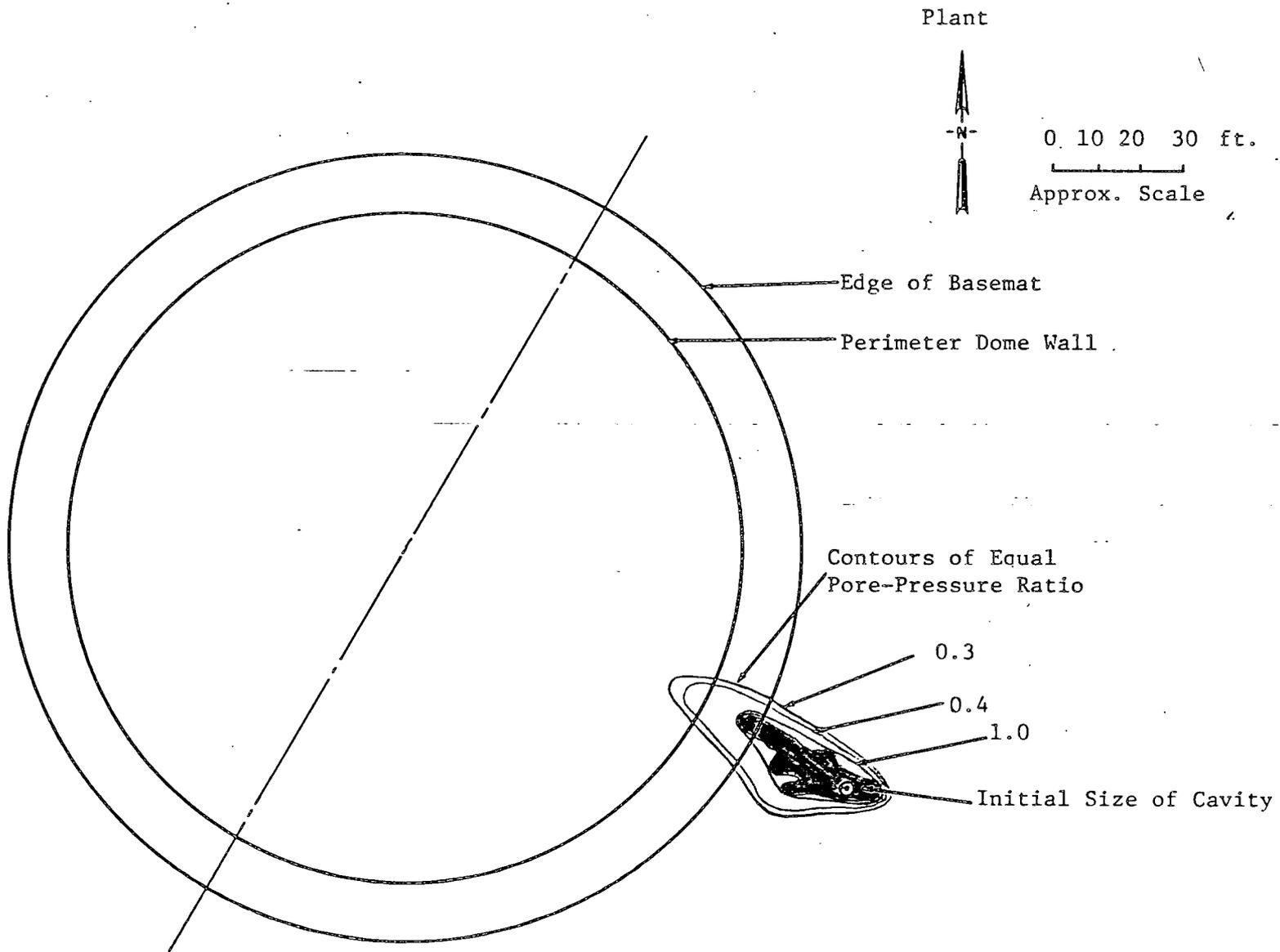
Fig. 7 SUMMARY OF RESULTS OF THE RESPONSE/PORE-PRESSURE DISSIPATION ANALYSIS - PLAN SECTION AT THE BASE OF THE TENDON GALLERY AND TIME = 12 SECS.
