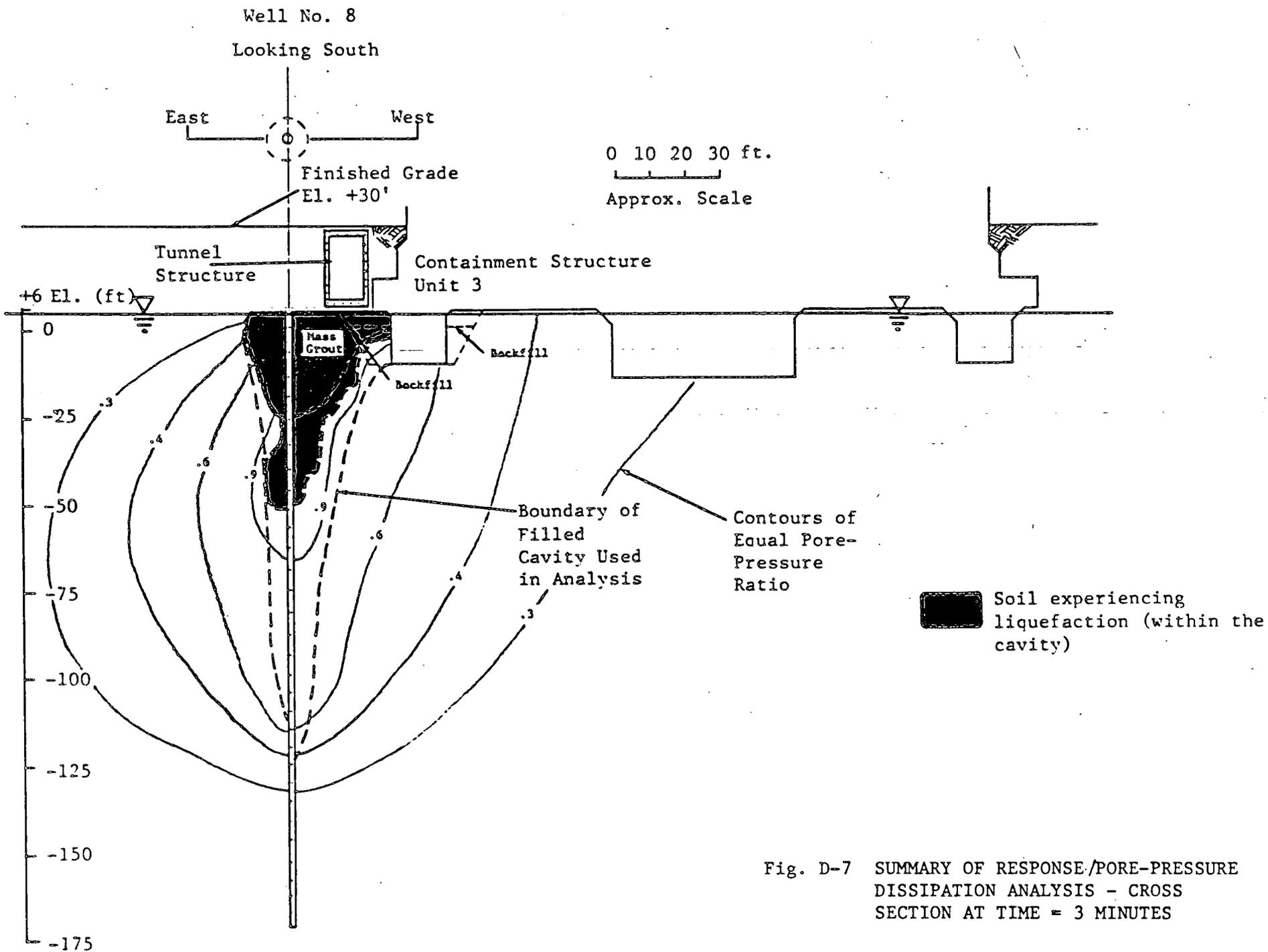
Fig. D-7 SUMMARY OF RESPONSE/PORE-PRESSURE DISSIPATION ANALYSIS - CROSS SECTION AT TIME = 3 MINUTES
