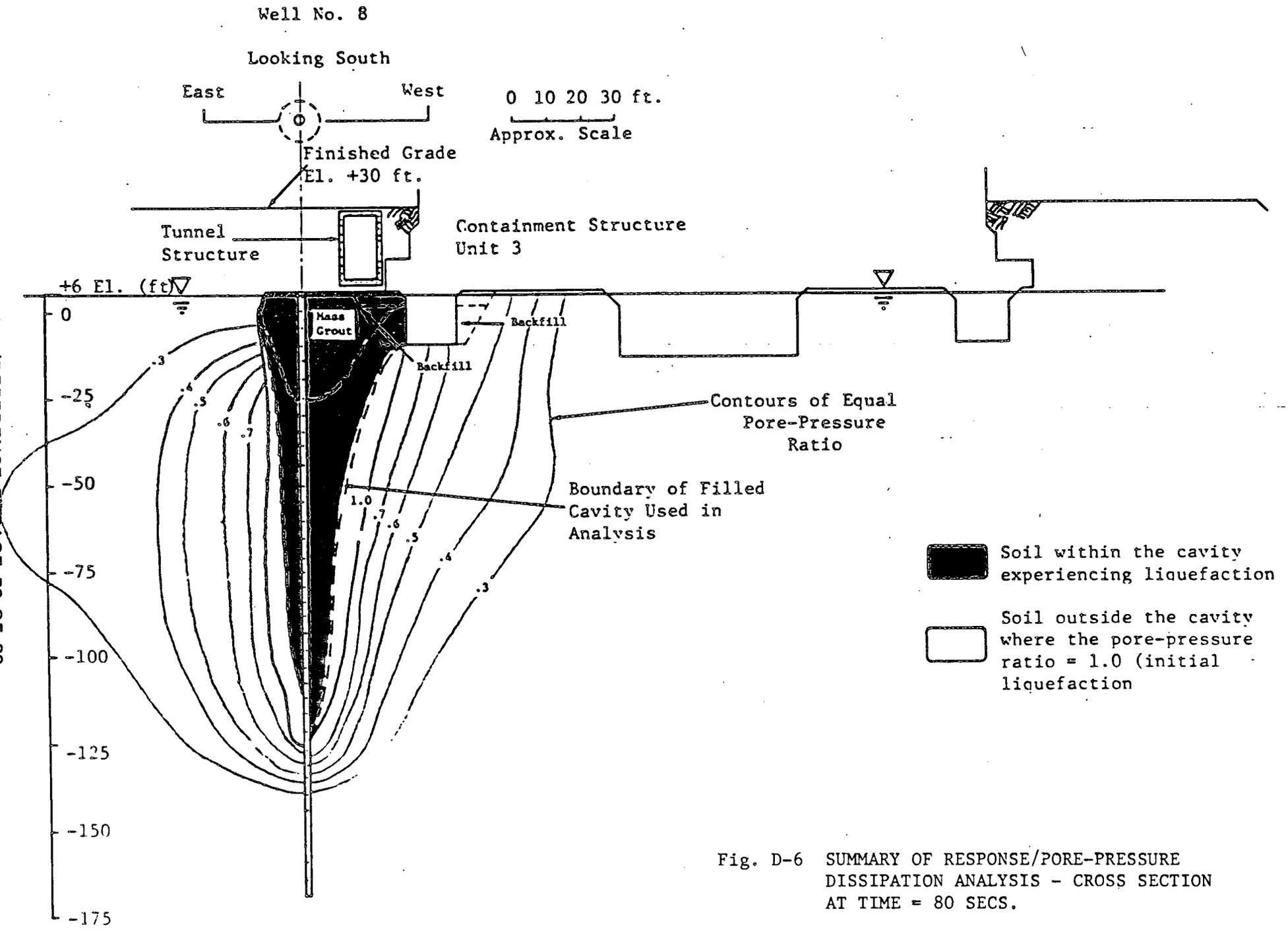
Fig. D-6 SUMMARY OF RESPONSE/PORE-PRESSURE DISSIPATION ANALYSIS - CROSS SECTION AT TIME = 80 SECS.
