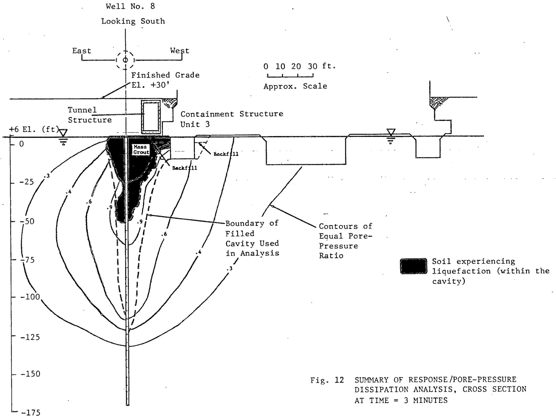
Fig. 12 SUMMARY OF RESPONSE/PORE-PRESSURE DISSIPATION ANALYSIS, CROSS SECTION AT TIME = 3 MINUTES
