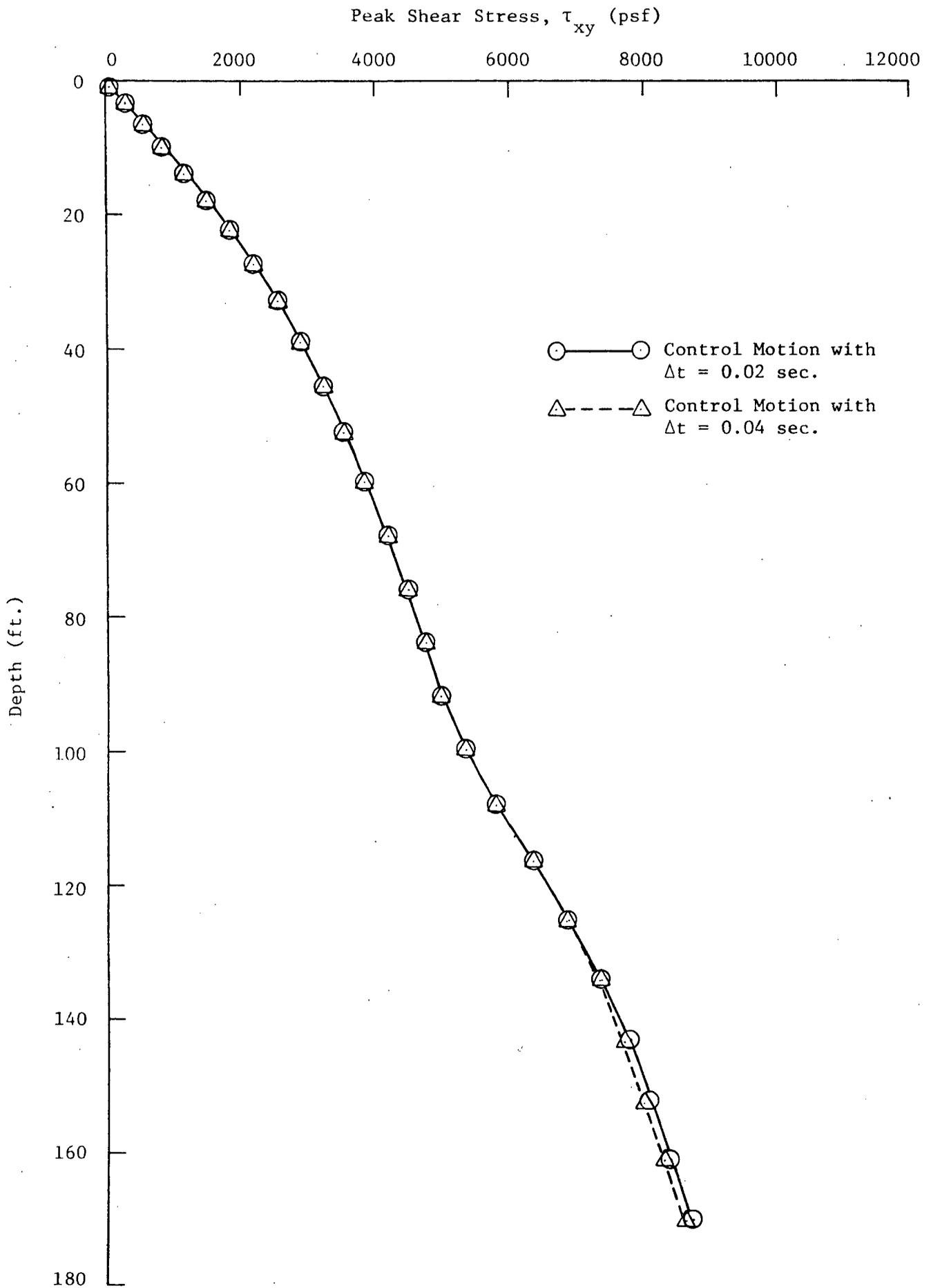
Fig. C-2 COMPARISONS OF PEAK SHEAR STRESSES FROM SHAKE ANALYSES USING DBE CONTROL MOTION WITH  $\Delta t = 0.02$  and  $0.04$  SECOND
