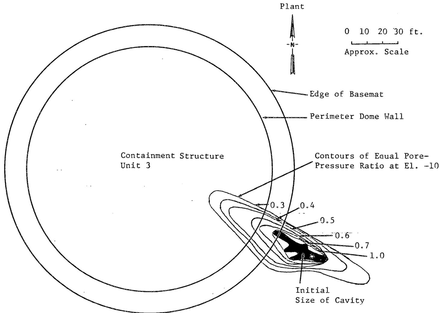
Fig. 9 SUMMARY OF THE RESULTS OF THE RESPONSE/PORE-PRESSURE DISSIPATION ANALYSIS -
