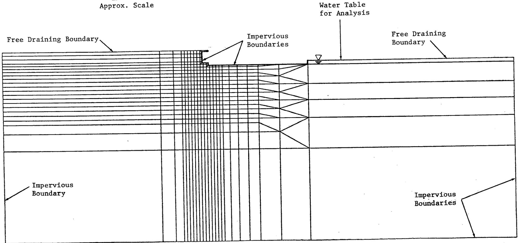
Fig. D-1 FINITE ELEMENT MESH FOR PLANE STRAIN ANALYSIS
