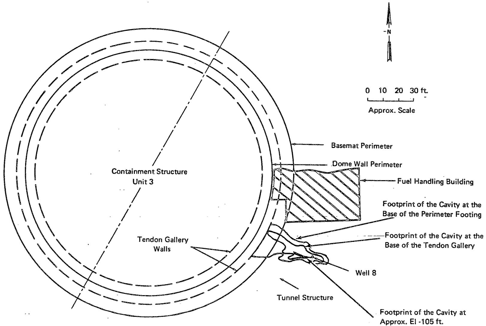
Fig. 2a INTERPRETED PLAN SECTIONS OF THE CAVITY AND THE CONTAINMENT STRUCTURE UNIT 3
