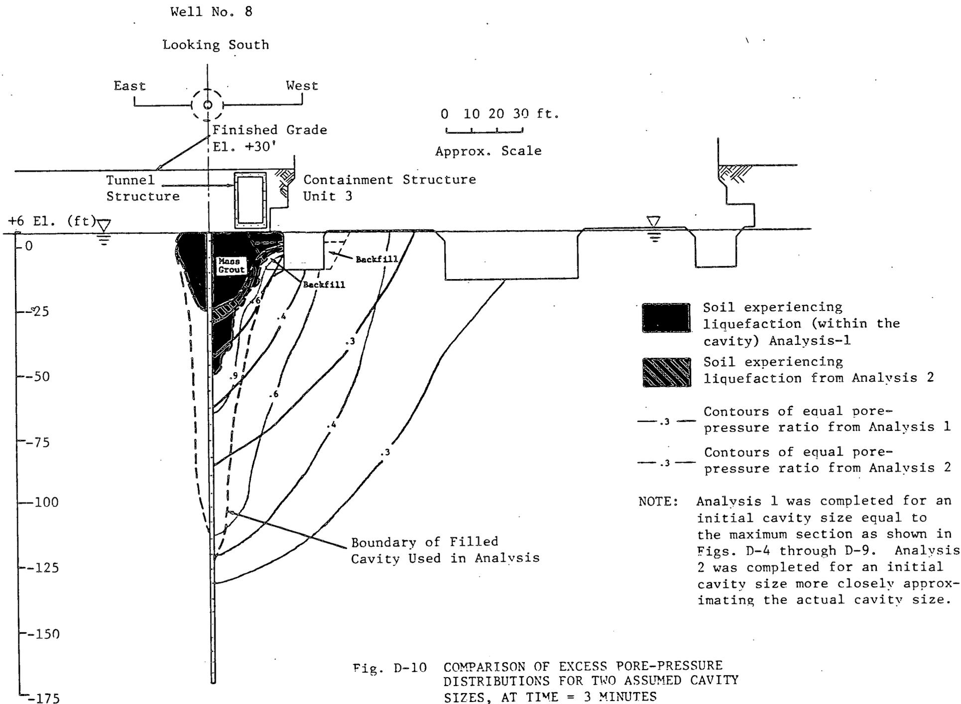
Fig. D-10 COMPARISON OF EXCESS PORE-PRESSURE DISTRIBUTIONS FOR TWO ASSUMED CAVITY SIZES, AT TIME = 3 MINUTES
