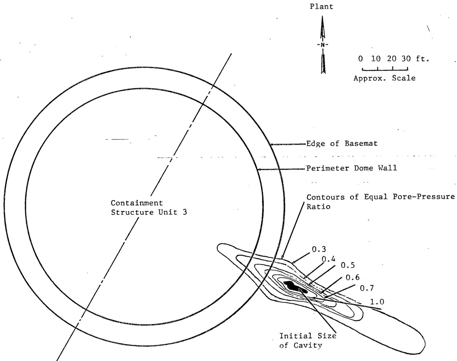
Fig. 10 SUMMARY OF RESULTS OF THE RESPONSE/PORE-PRESSURE DISSIPATION ANALYSIS - FOR EL. -60 AND TIME = 80 SECS.
