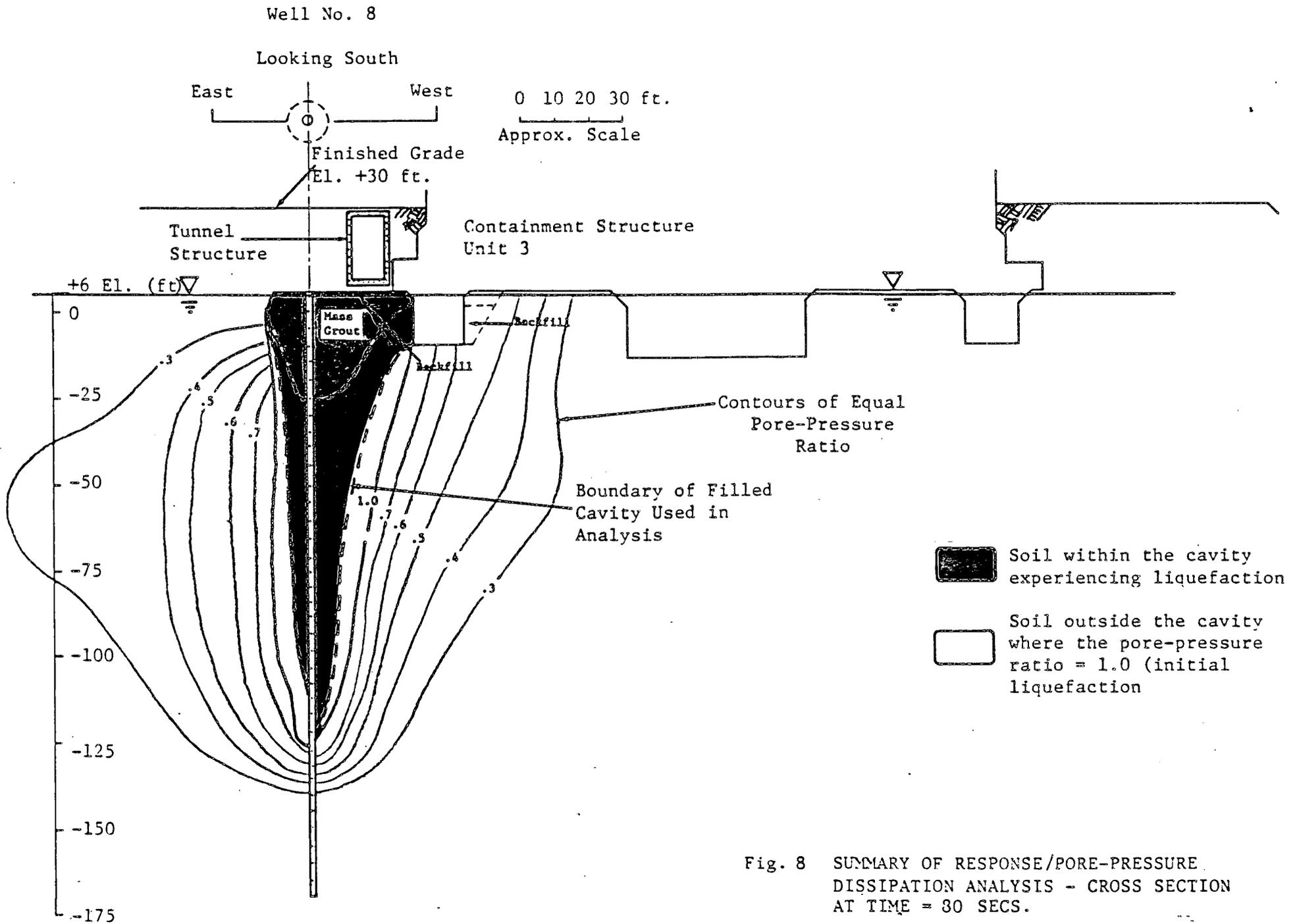
Fig. 8 SUMMARY OF RESPONSE/PORE-PRESSURE DISSIPATION ANALYSIS - CROSS SECTION AT TIME = 30 SECS.
