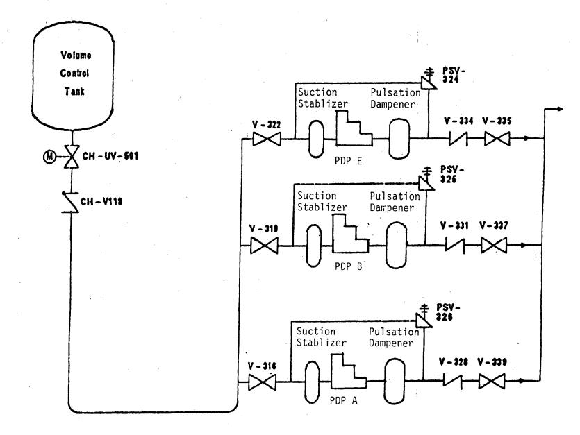
Figure 1. Charging Pumps at Palo Verde Units 1 and 2.
