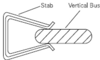
**Figure 1 Sketch of Stab & Vertical Electrical Bus**
