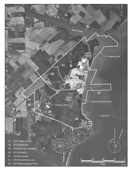
**Figure 3-2**. Fermi Site Layout Showing Existing and Proposed Facilities: Ancillary Facilities (Detroit Edison 2011b)
