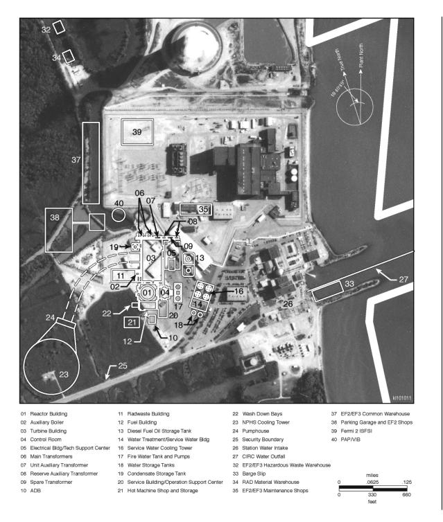
**Figure 3-1**. Fermi Site Layout Showing Existing and Proposed Facilities: Power Block and Adjacent Facilities (Detroit Edison 2011b)
