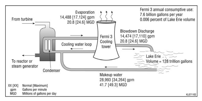
Figure 5-1. Fermi 3 Water Use Diagram
