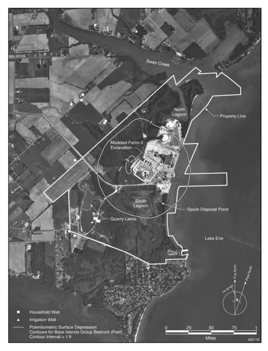
**Figure 4-2**. Modeled Drawdown of Groundwater in the Bass Islands Group as a Result of Dewatering for Fermi 3 Construction – Scenario 1 (Detroit Edison 2011a)
