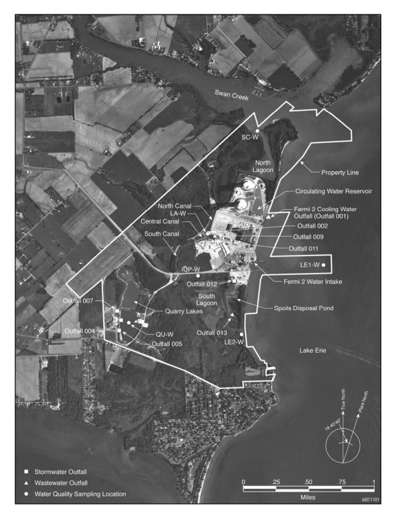
**Figure 2-6**. Surface Water Features, Discharge Outfalls, and Water Quality Sampling Locations on the Fermi Site
