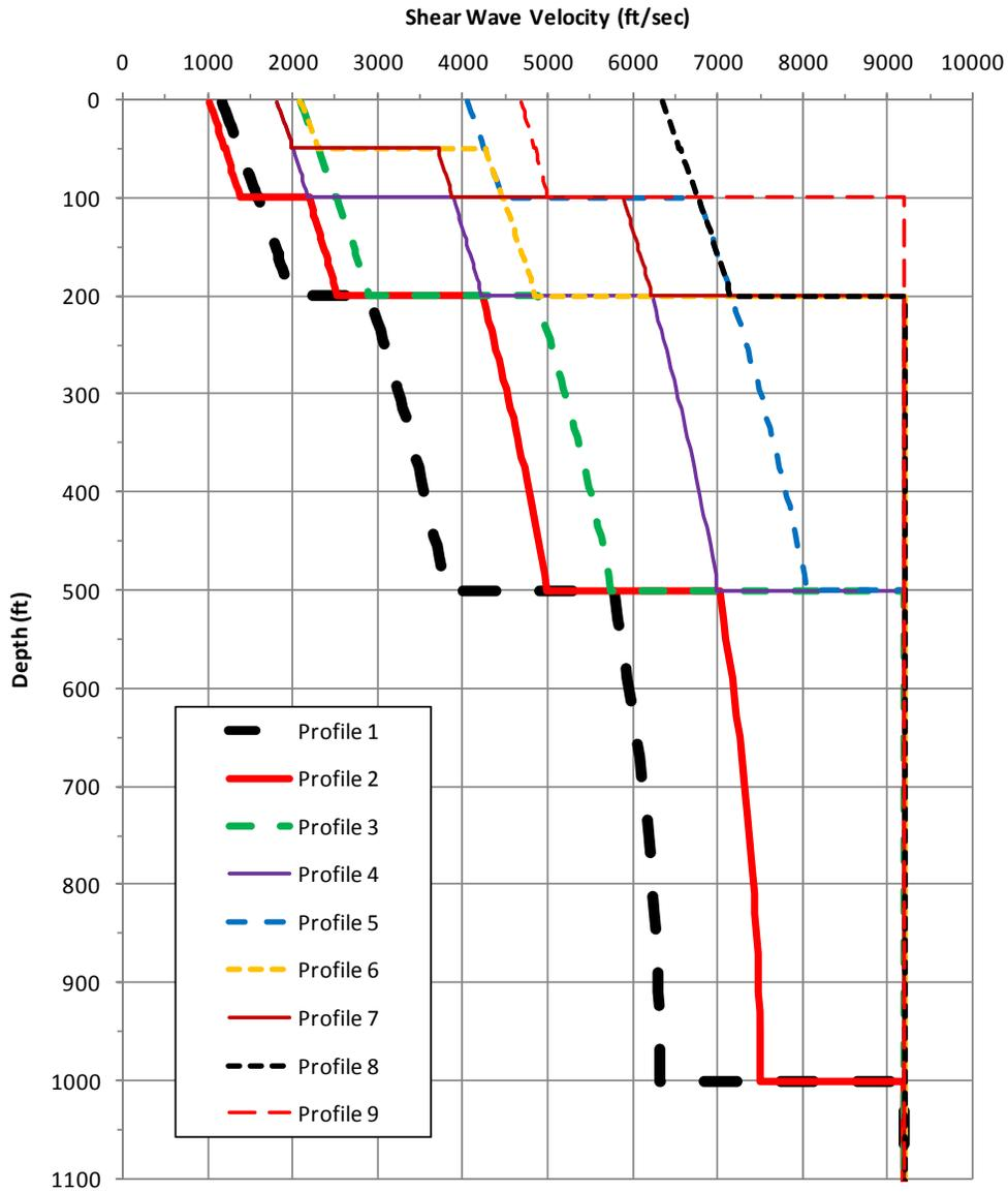
Figure 3-6. Low-Strain Shear Wave Velocity Profiles vs.. Depth for the Nine Generic Site Profiles Considered for APR1400
