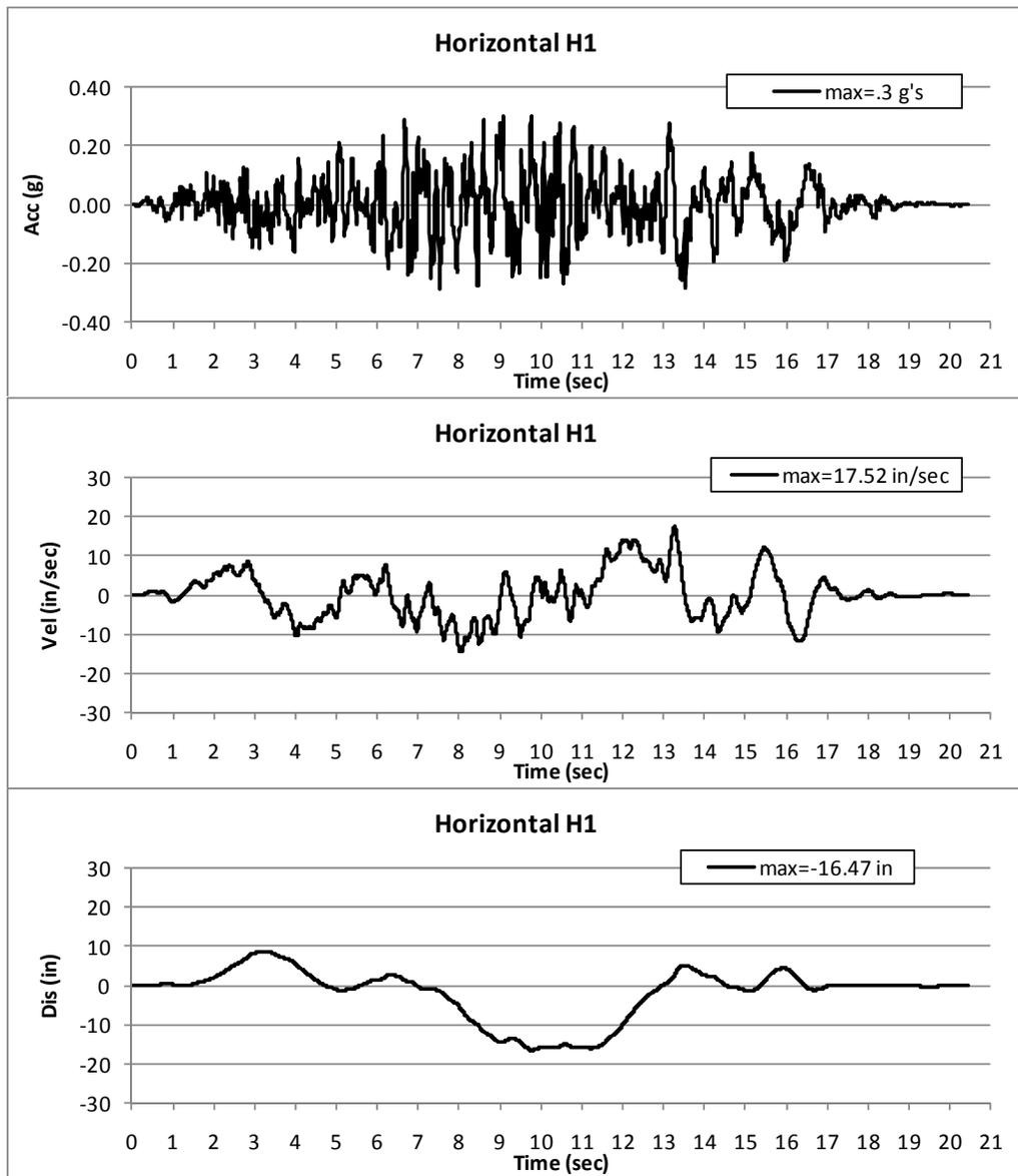
Figure 3-3. CSDRS-Compatible Design Acceleration, Velocity, and Displacement Time Histories - H1 Component
