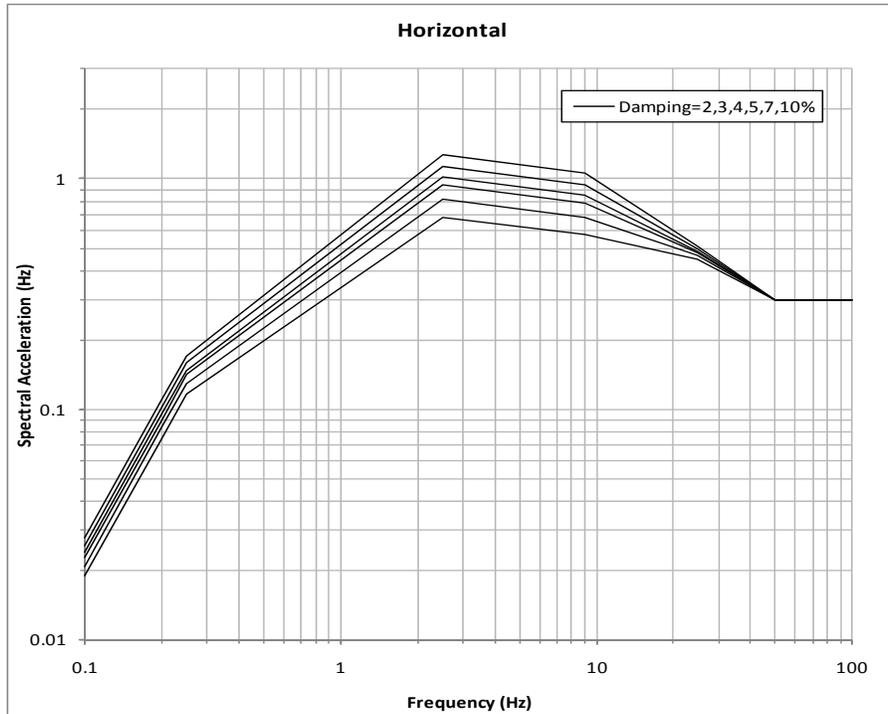
Figure 3-1. APR1400 Horizontal Certified Seismic Design Response Spectra (CSDRS)
