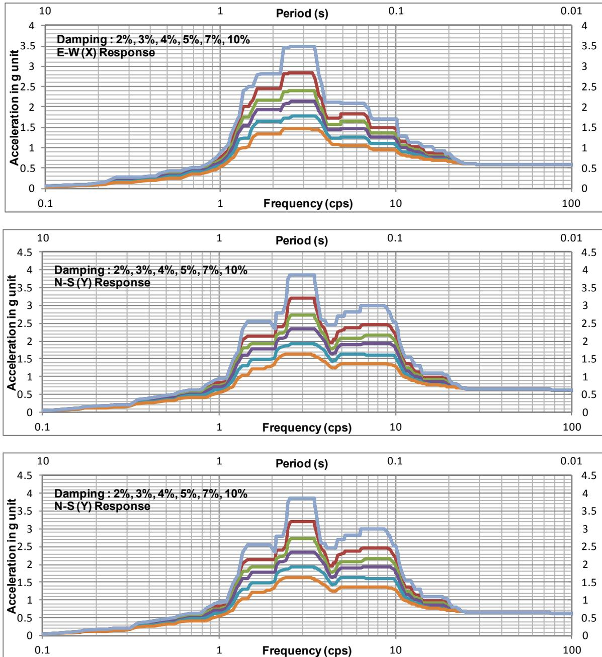
Figure 4-10. ISRS at AB El.156'-0" for Individual SSI Analysis (Surface Structure) S1U
