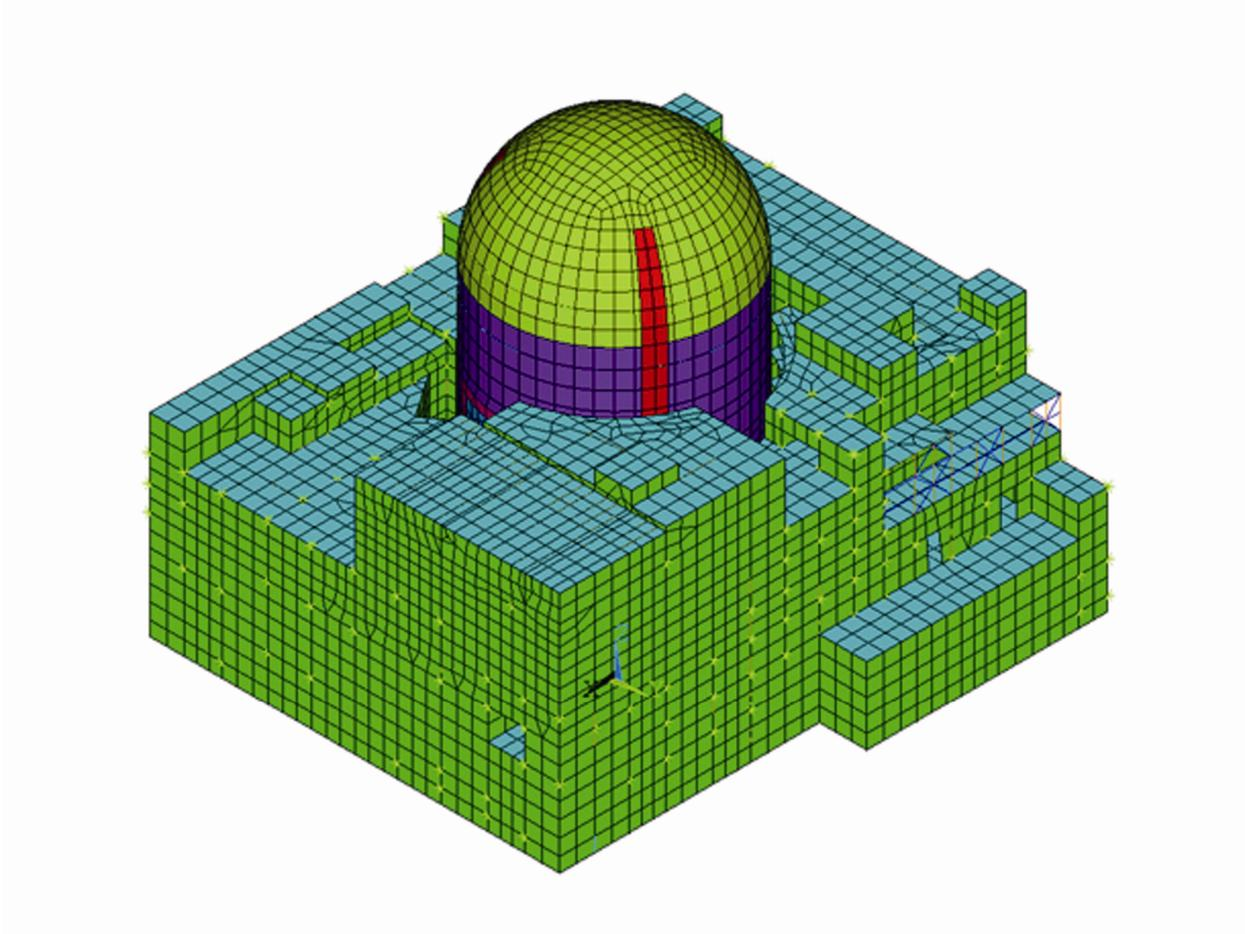
Figure 4-2. Combined SASSI SSI Finite Element Model of Nuclear Island
