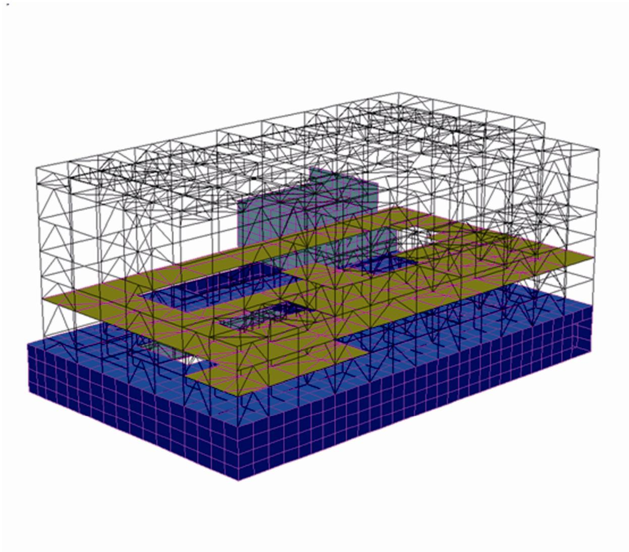
Figure 4-5. SASSI SSI Finite Element Model of Turbine Island
