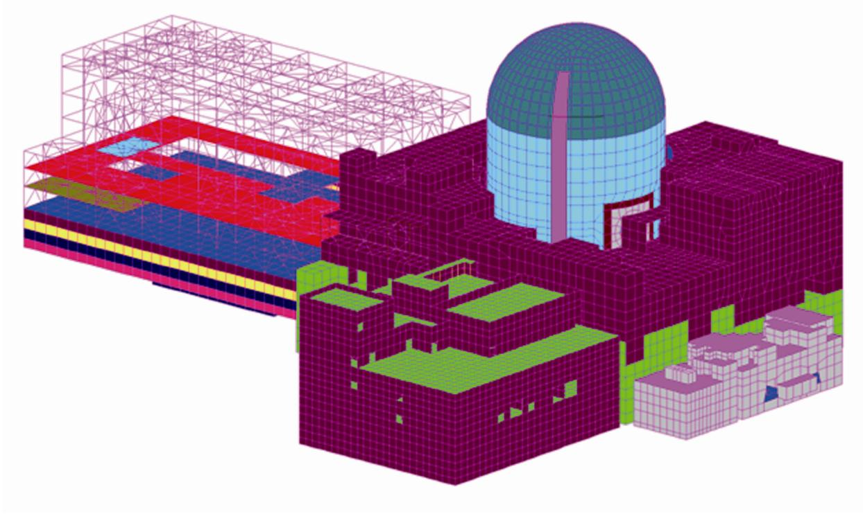
Figure 4-6. SASSI SSSI Finite Element Model of Power Block
