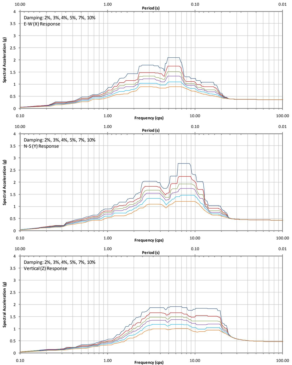
Figure 4-7. ISRS at AB El.156'-0" for Design Basis SSI Analysis (Embedded Structure) S1U
