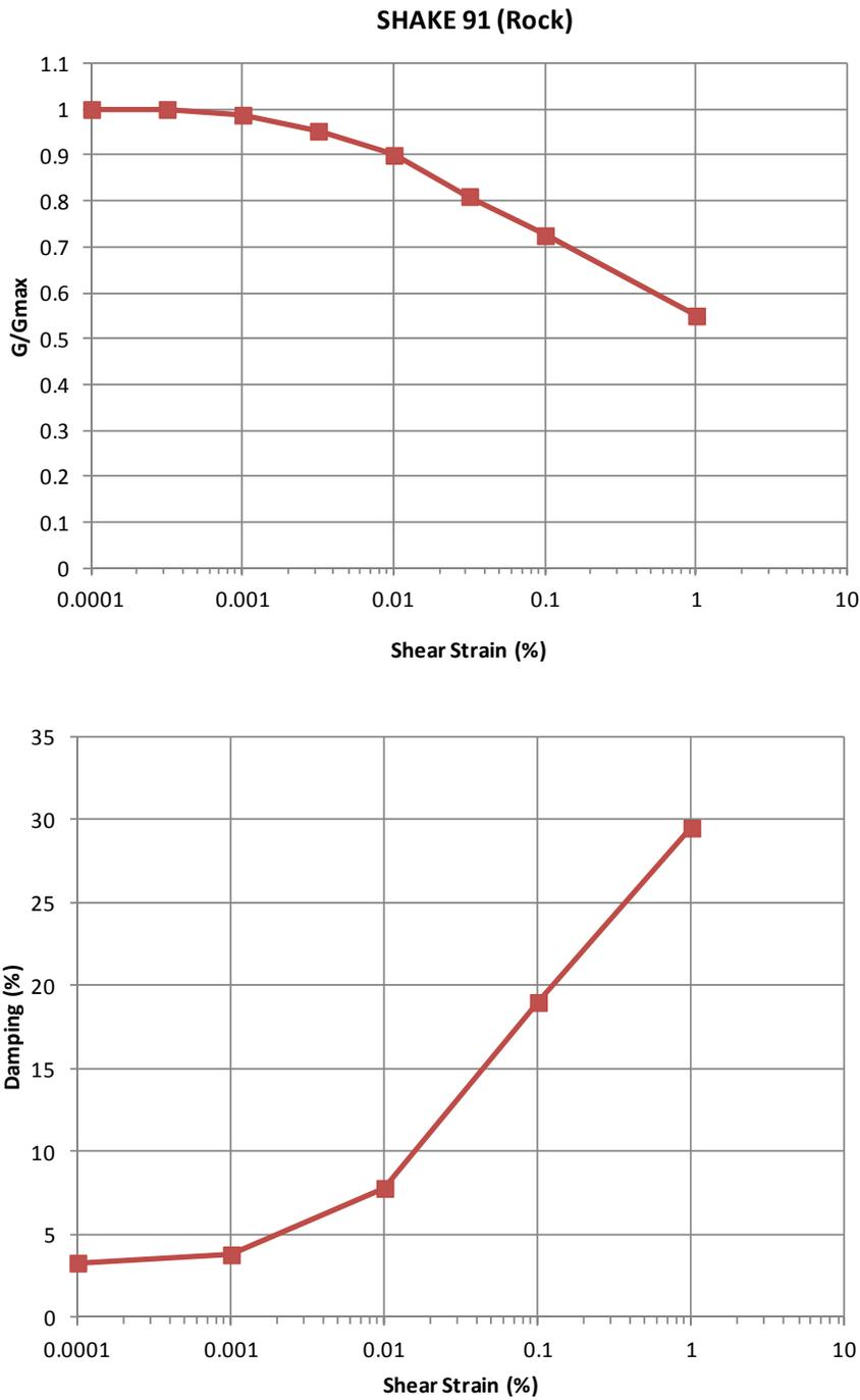
Figure 3-9. Shear-Modulus-Degradation and Damping-Value Variation Curves for Rock Considered for APR1400
