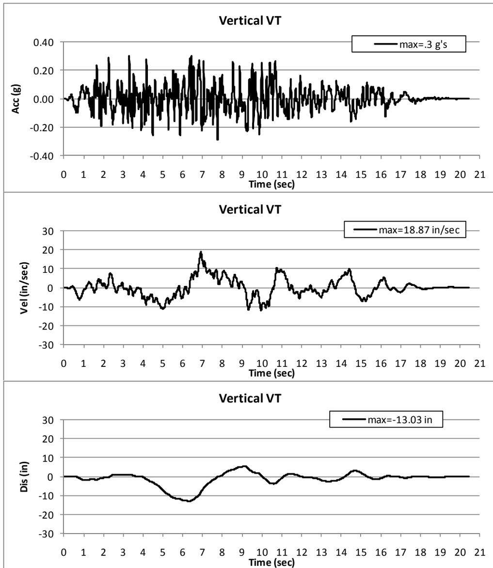
Figure 3-5. CSDRS-Compatible Design Acceleration, Velocity, and Displacement Time Histories - VT Component
