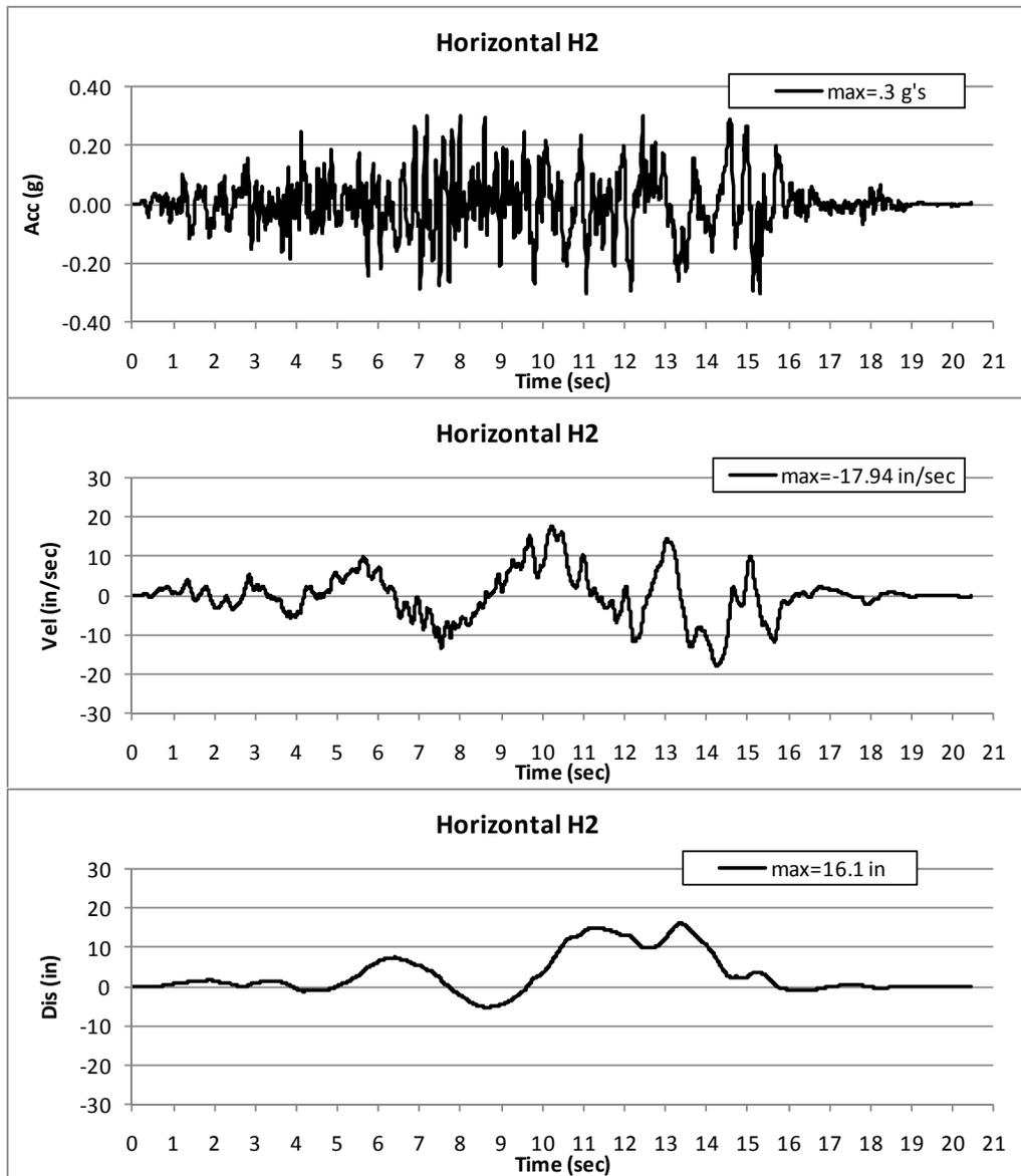
Figure 3-4. CSDRS-Compatible Design Acceleration, Velocity, and Displacement Time Histories - H2 Component
