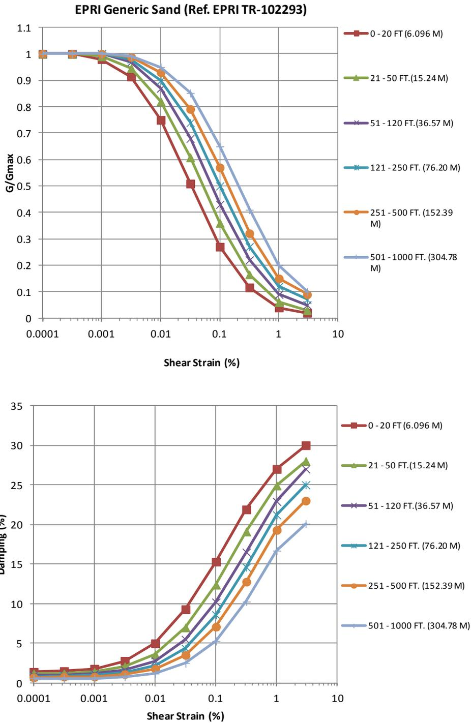
Figure 3-7. Shear-Modulus-Degradation and Damping-Value Variation Curves for Sand Considered for APR1400
