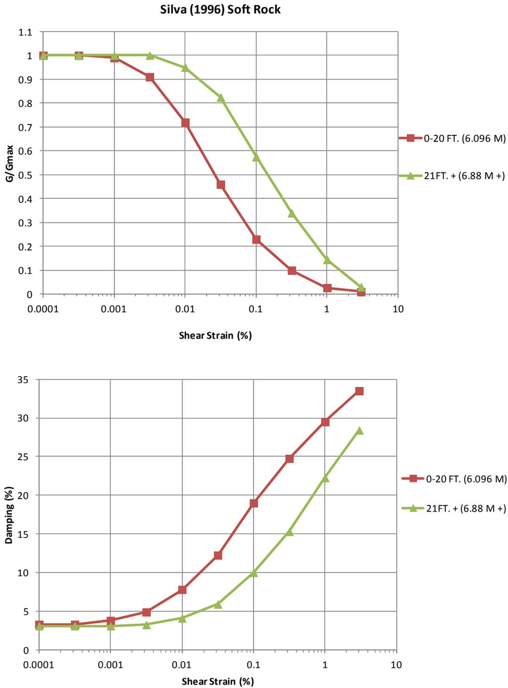
Figure 3-8. Shear-Modulus-Degradation and Damping-Value Variation Curves for Soft Rock Considered for APR1400
