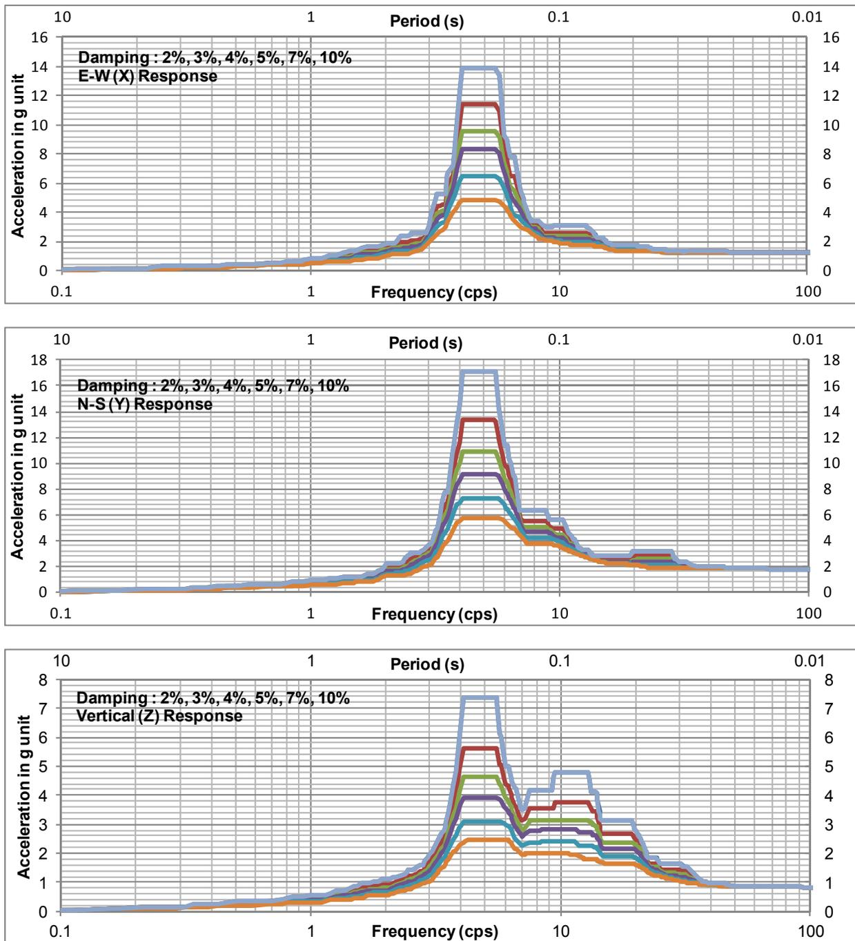
Figure 4-12. ISRS at AB El.156'-0" for Individual SSI Analysis (Surface Structure) S9U
