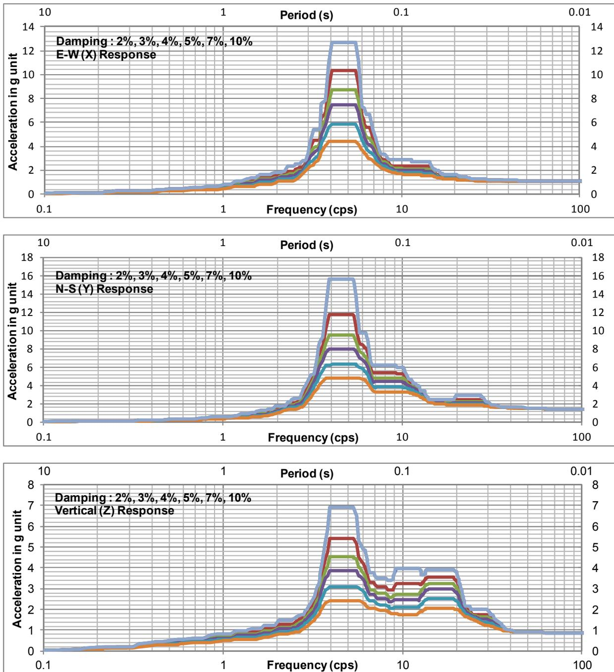
Figure 4-11. ISRS at AB El.156'-0" for Individual SSI Analysis (Surface Structure) S5U
