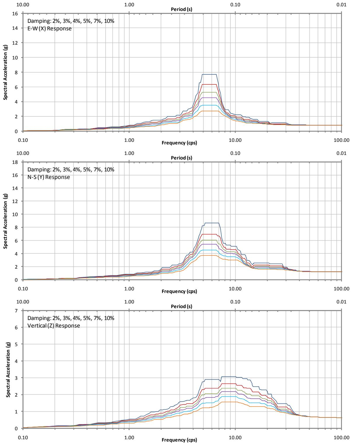
Figure 4-8. ISRS at AB El.156'-0" for Design Basis SSI Analysis (Embedded Structure) S5U
