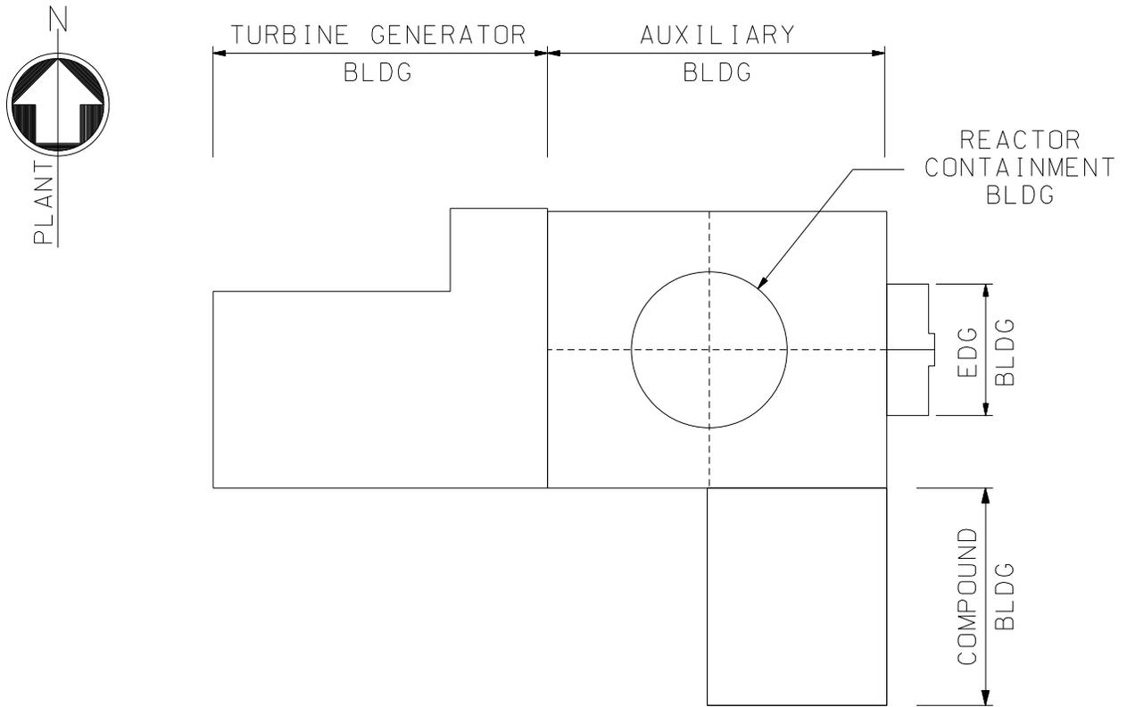
Figure 2-1. Plan Layout of APR1400 Power Block
