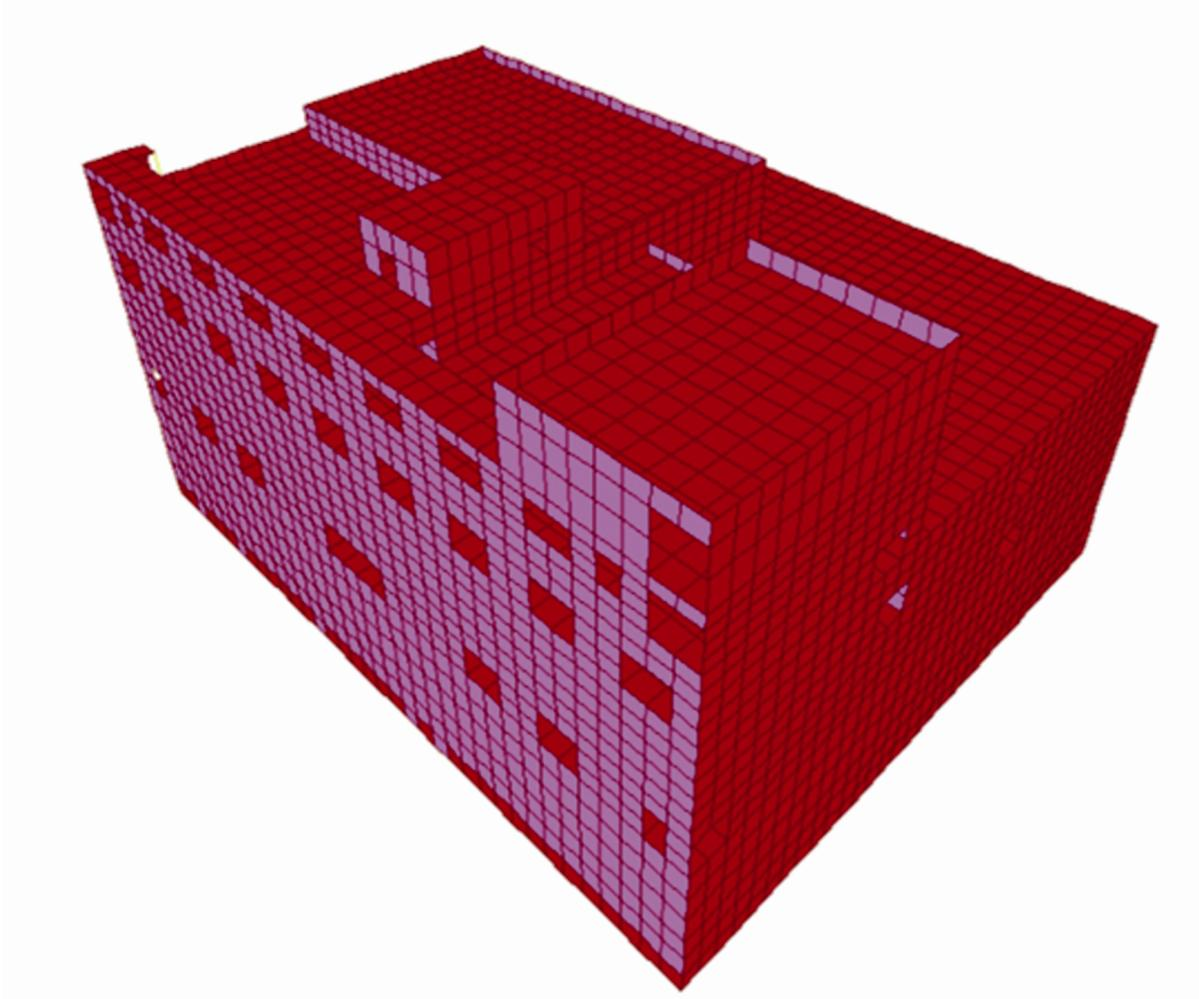
Figure 4-4. SASSI SSI Finite Element Model of Compound Building
