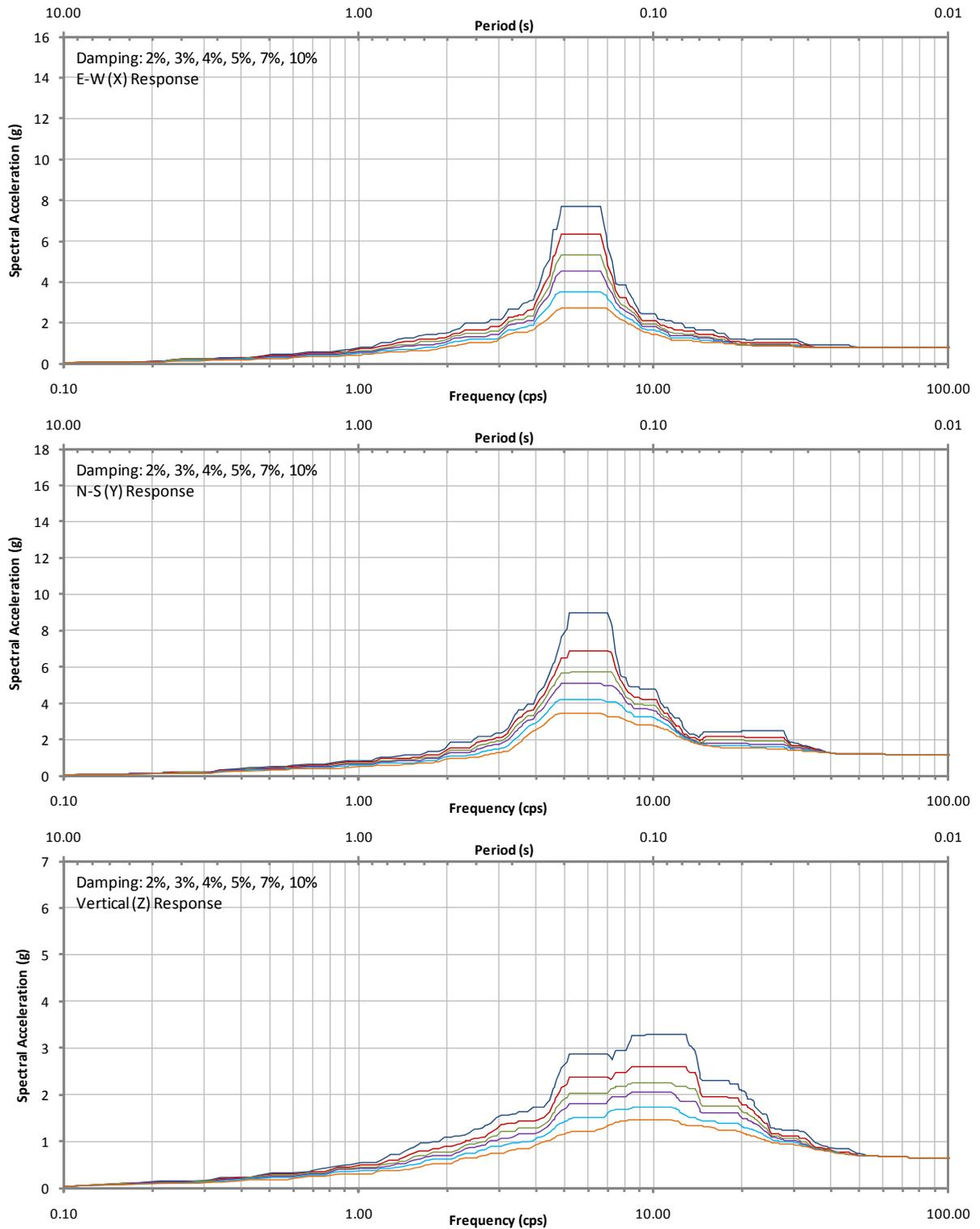
Figure 4-9. ISRS at AB El.156'-0" for Design Basis SSI Analysis (Embedded Structure) S9U
