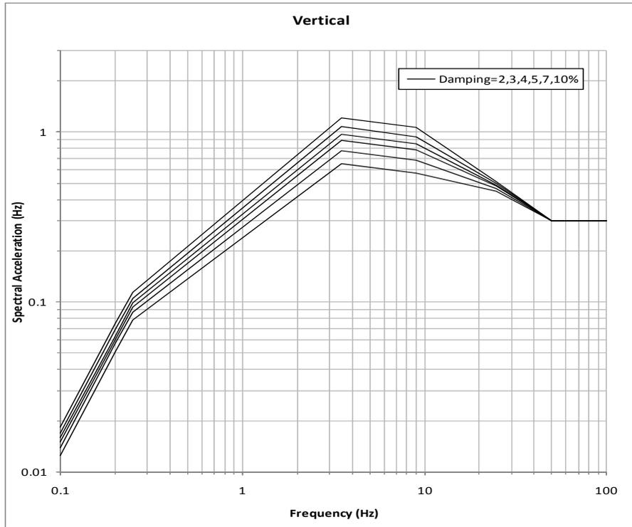
Figure 3-2. APR1400 Vertical Certified Seismic Design Response Spectra (CSDRS)
