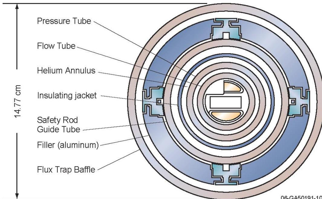
**Figure 3-3 Cross section of the in-core portion of a typical pressurized water loop**
