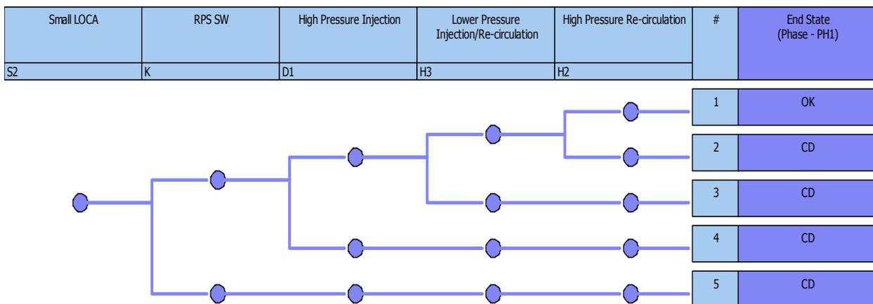
**Figure 5-1 Integrating software into PRA: a small LOCA example**
