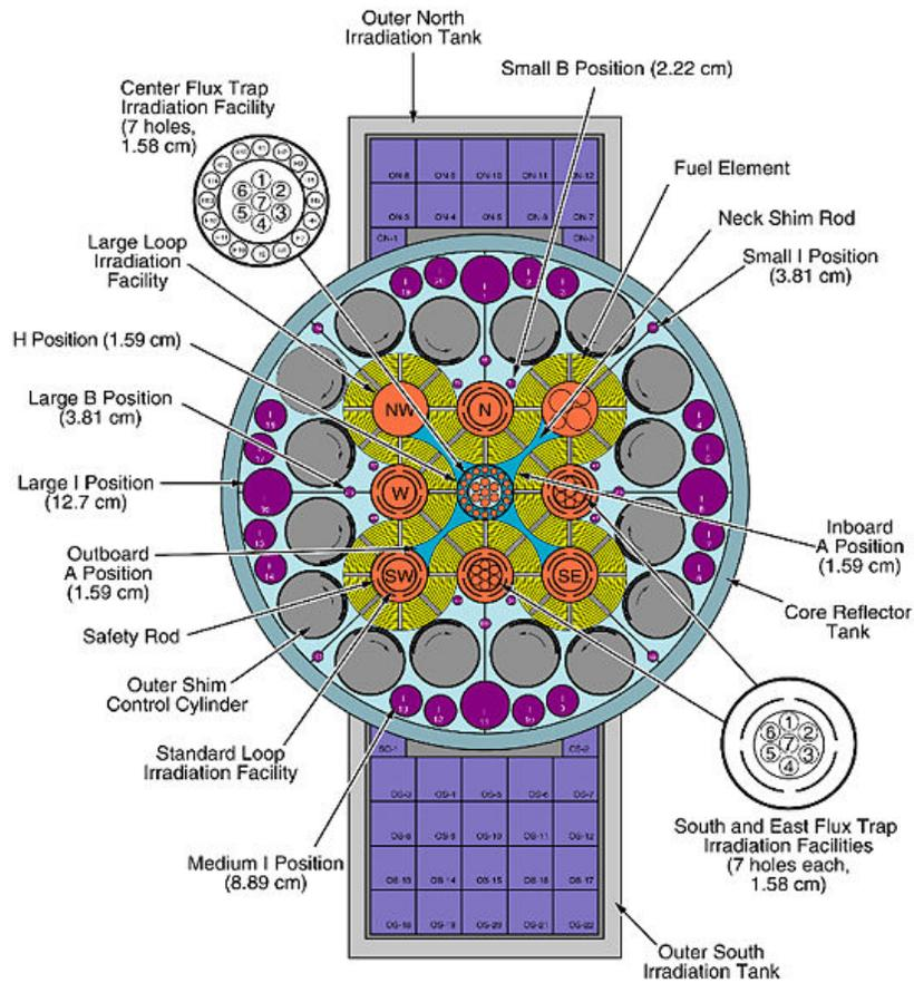
**Figure 3-2 Core cross section of Advanced Test Reactor**
