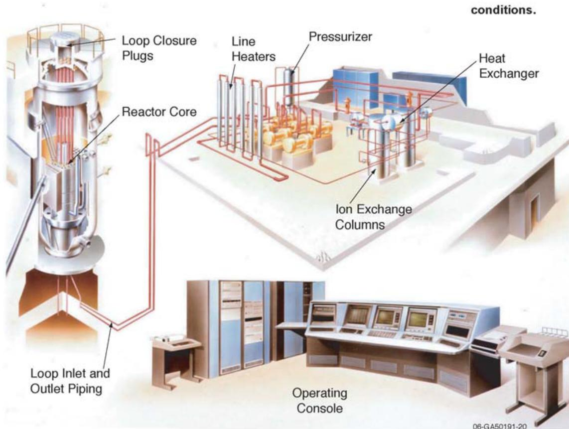
**Figure 3-4 Pressurized water loop system**
