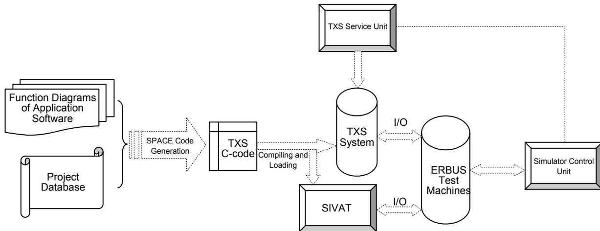
**Figure A-1 ERBUS TELEPERM XS concept**
