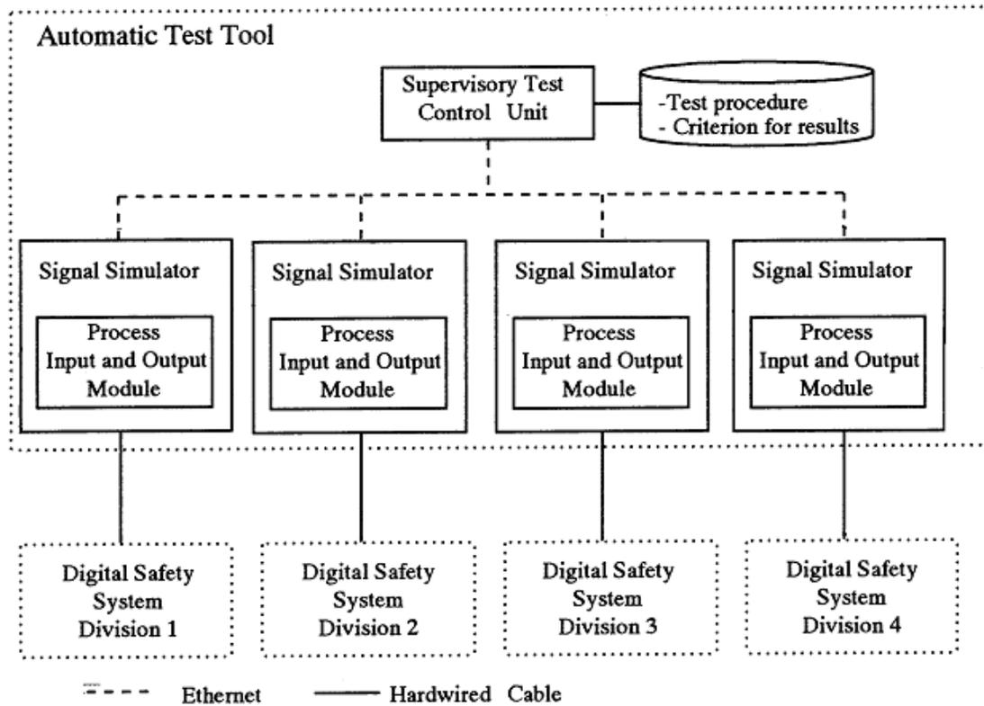
**Figure A-2 Test configuration of an ABWR**
