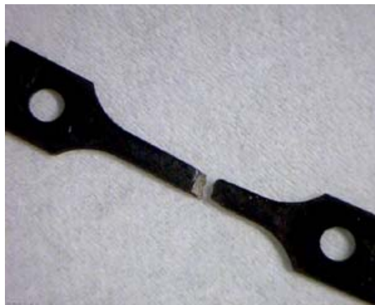
Figure 4. A BOR-60 sample tested in the simulated PWR environment.
