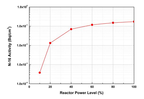
Figure 11B-1 N-16 Concentrations with Power at SG Leakage of 4.73 L/hr (30 gpd)
