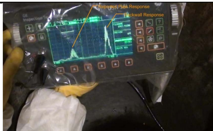
0° Conventional UT, Safety Nozzle A
