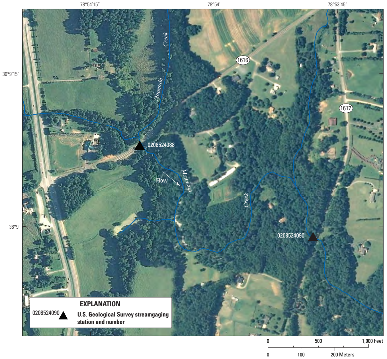
Figure 21. Plan view of Mountain Creek channel configuration and location of streamflow-gaging and sampling sites near Bahama, North Carolina.
