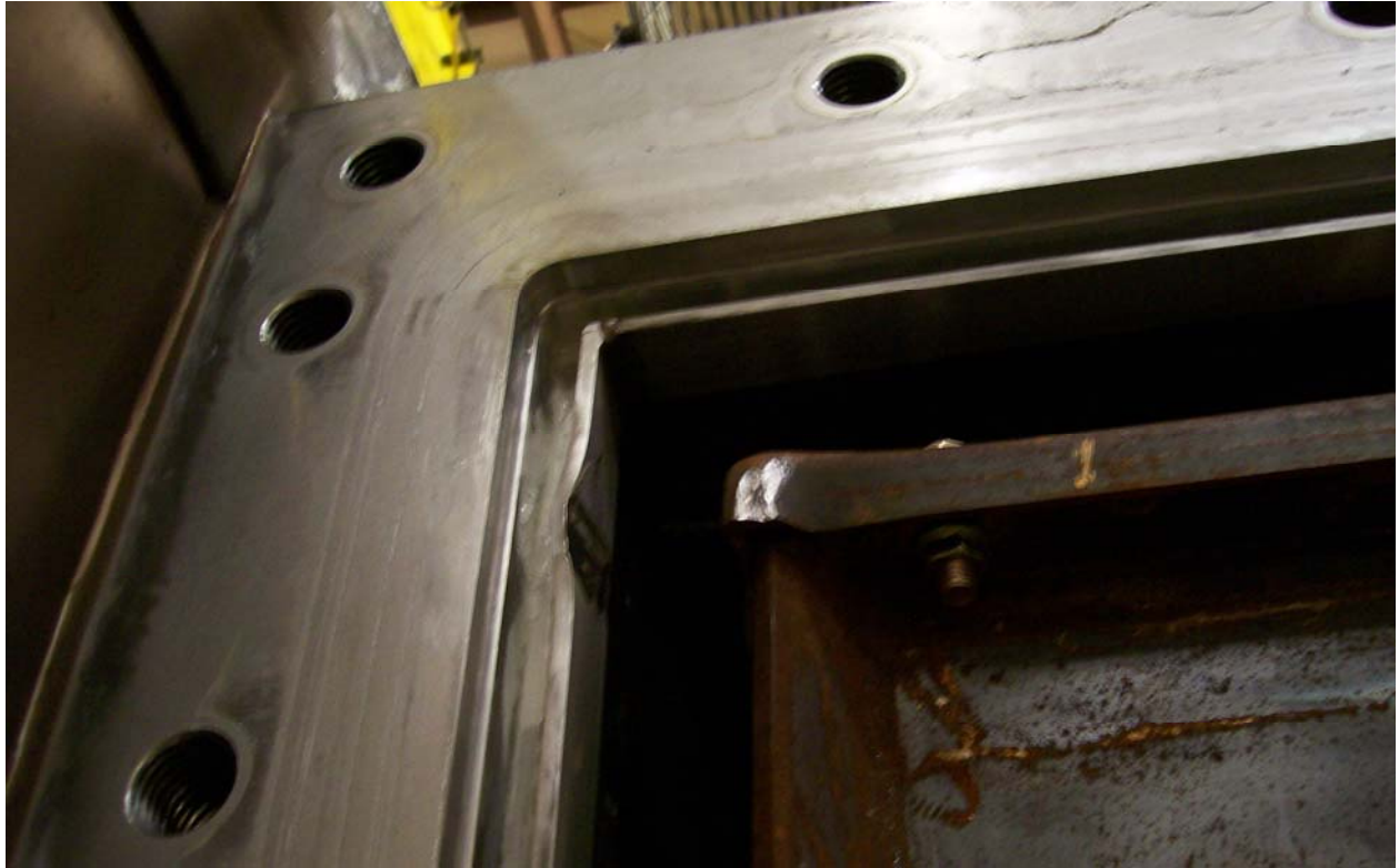
Figure 2.12.6-19 – Dent in Debris Shield Receptacle Caused by SLB2
