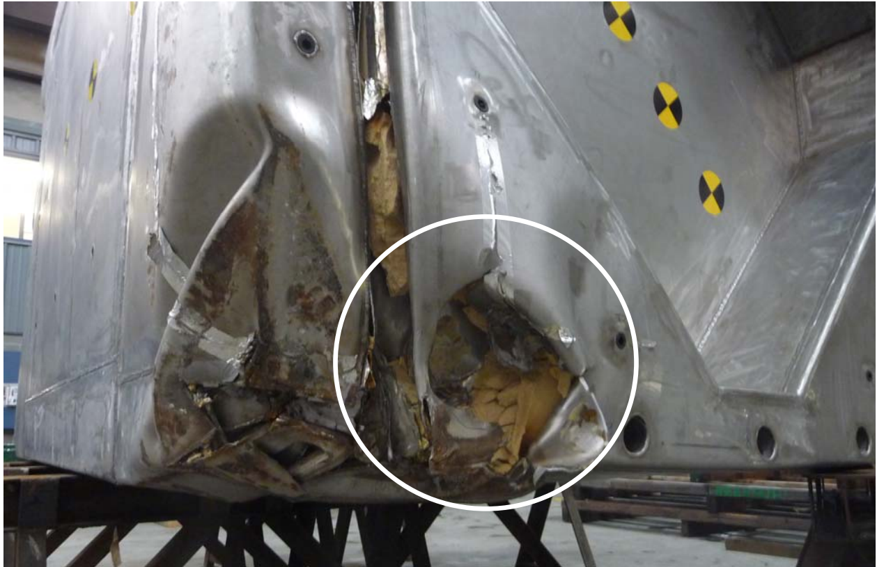
Figure 2.12.6-13 – Test LP91, CG-Over-Corner Puncture Damage
