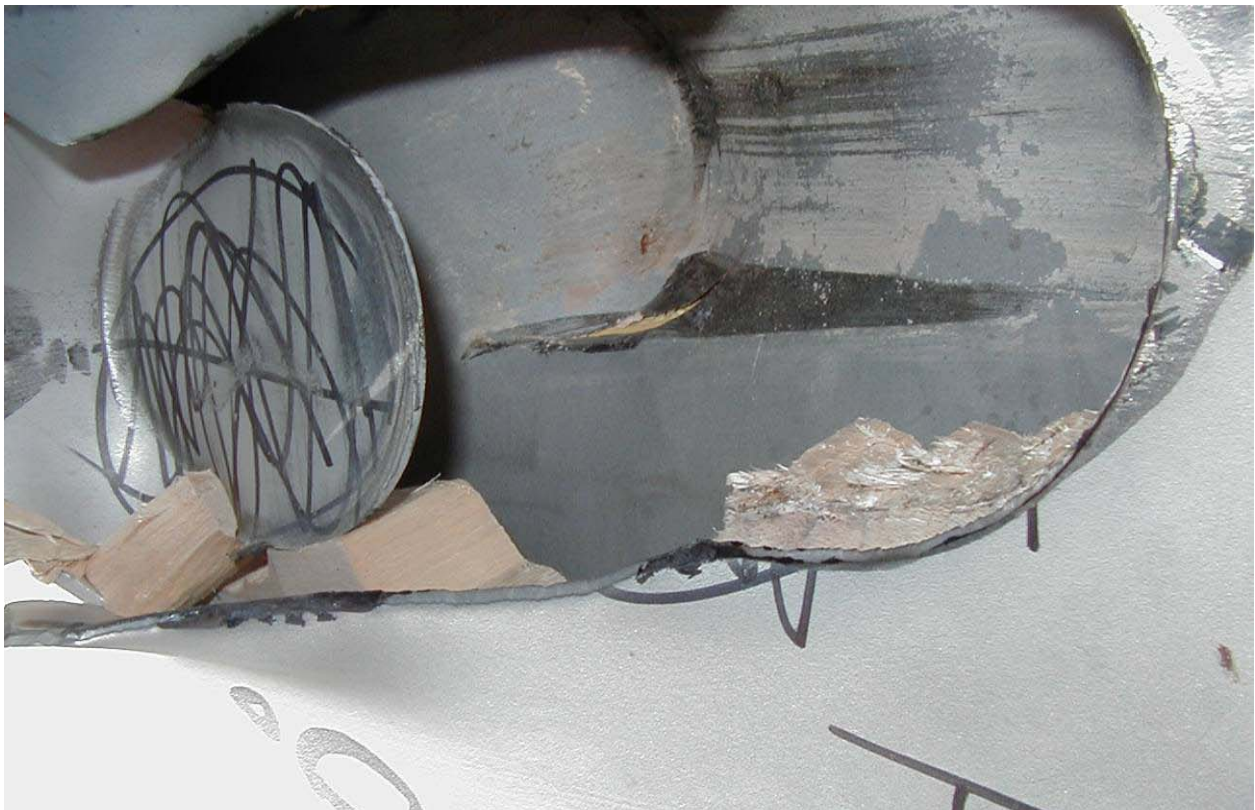
Figure 2.12.1-58 – Puncture Drop Test P205 at 30°
