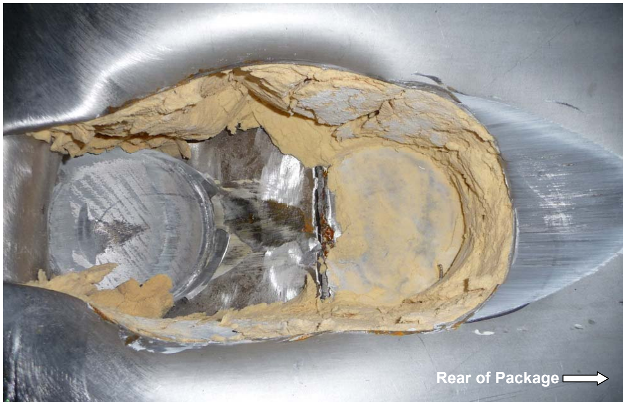
Figure 2.12.6-15 – Test LP92, Puncture on Bottom Wall Damage, Detail
