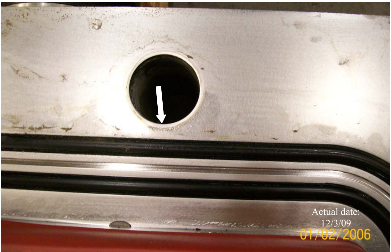
Figure 2.12.6-18 – Galling on Flange Around Closure Bolt Holes
