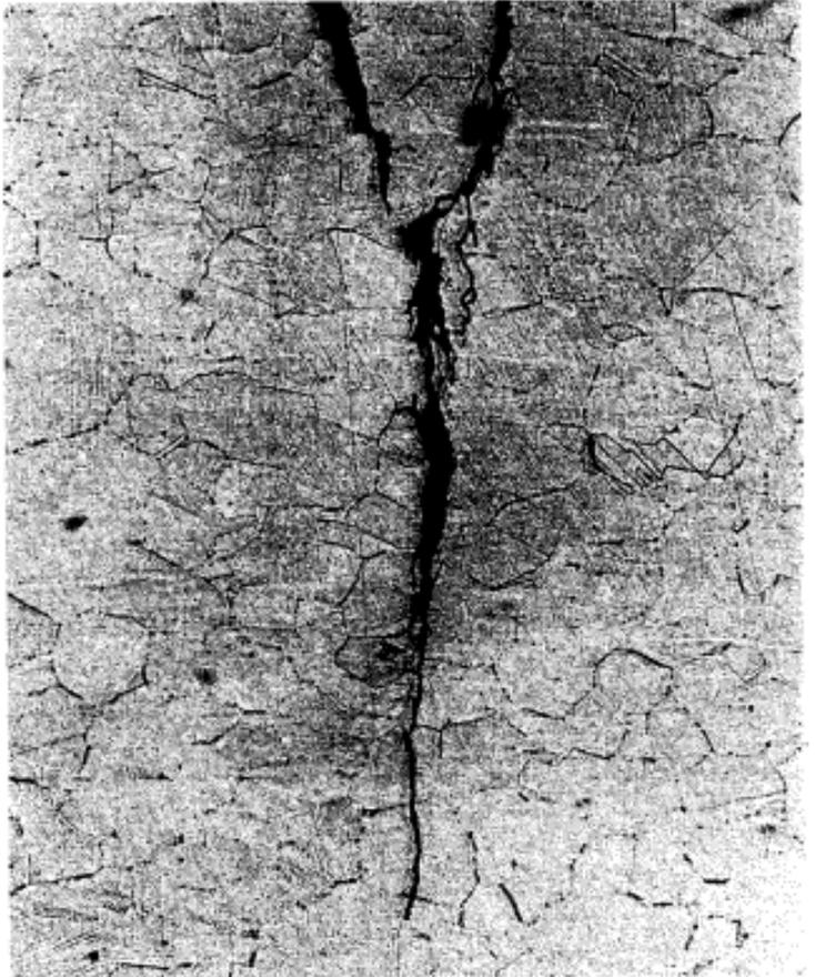
**Type 304 stainless steel piping contaminated with chlorides. Crack depth is about 1.2 mm (50 mils) (Stein, et al., 1986).
