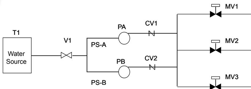
**Success Criteria:** Flow from any one pump through any one MV
