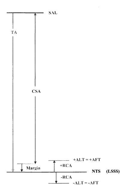
Figure 3-1 Westinghouse Setpoint Parameter Relationship Diagram (Increasing Function)
