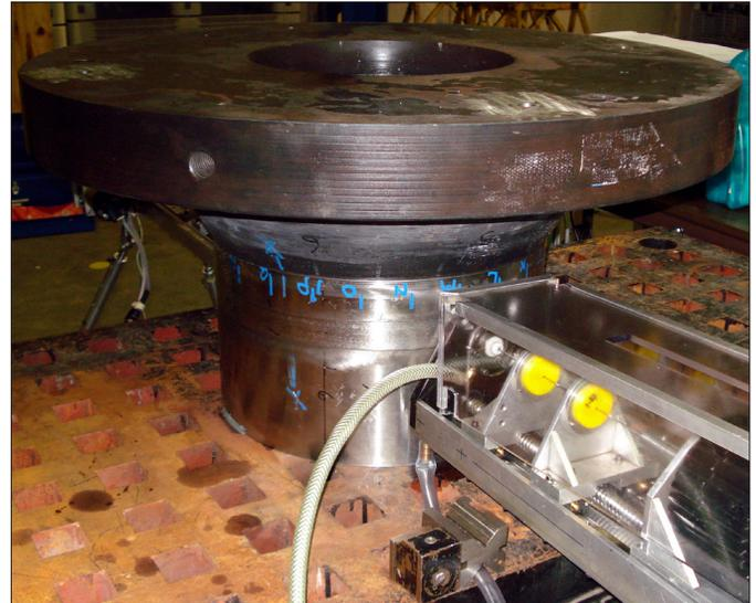
Figure 9.12 Pressurizer surge nozzle DM weld mockup being measured for WRSs
