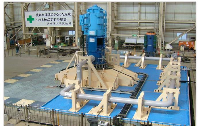
Figure 12.15 JNES seismic fragility test of large vertical shaft pump
