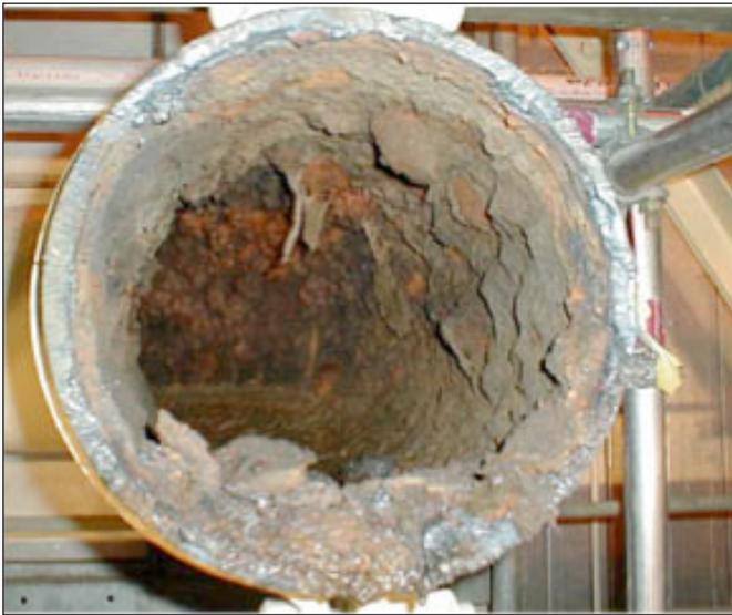
Figure 9.23 Corrosion and biofouling of carbon steel service water system piping
