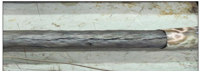
**Figure 7.13** Photo of Kerite-FR cable after testing, showing the cracking of insulation material
