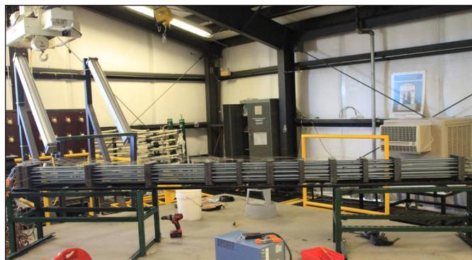
Figure 12.7 Single fuel assembly for Phase 1 testing in construction stage
