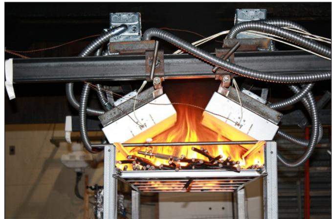
Figure 7.5 Radiant panel cable tray fire test (side view of burning cables in a tray exposed to a radiant heat source)
