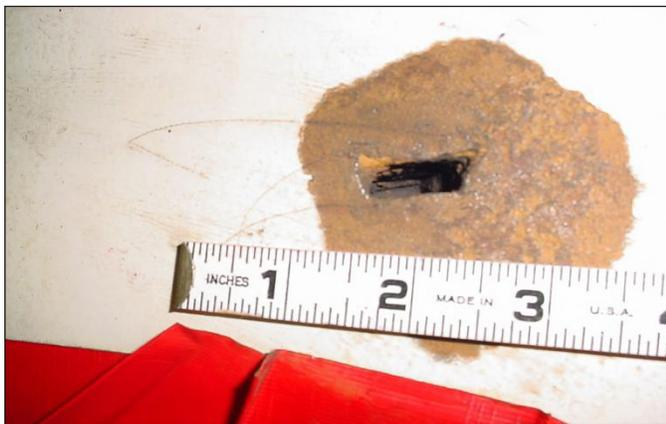
**Figure 9.18** Photograph of the through-wall corrosion detected at Beaver Valley, 2009. A piece of wood embedded in the concrete during original construction was found behind the corroded area of the steel containment liner. The area was identified by a large paint blister which was filled with steel corrosion products
