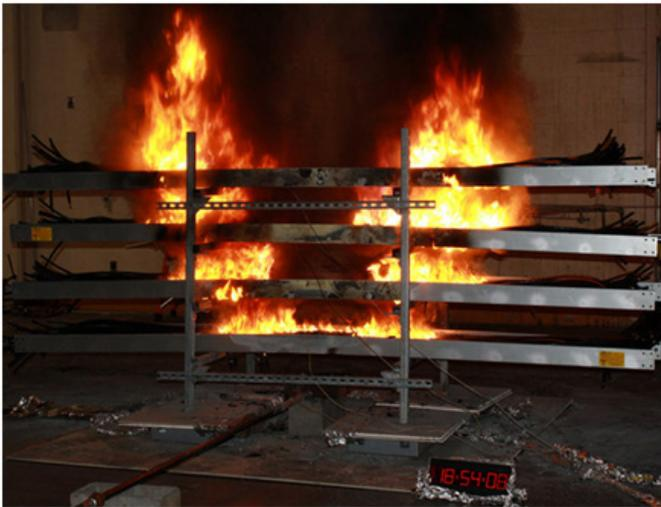
Figure 7.6 Burning cables during cable tray fire test (side view of burning cables in trays during a multiple-tray test after ignition using a small gas burner)
