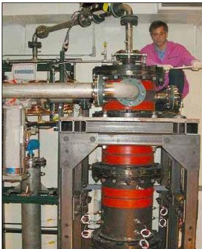
Figure 3.8 MCCI Experimental Setup
