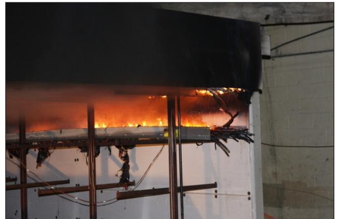
**Figure 7.8** Burning cables in hallway enclosure (end view of burning cables in two horizontal trays in hallway enclosure)
