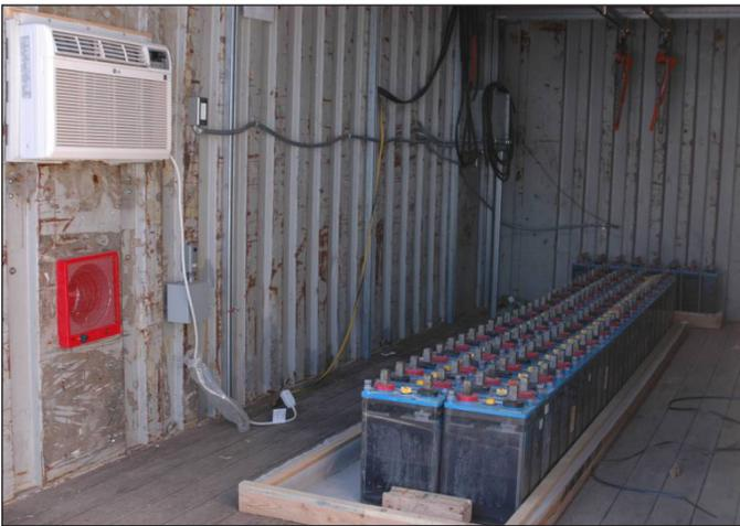
Figure 7.11 Battery bank for dc fire tests
