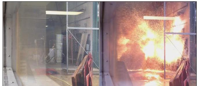
Figure 7.22 480 V load center undergoing HEAF testing: before arcing (left); after arcing (right)
