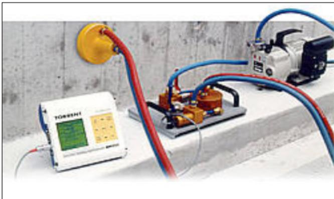
Figure 12.19 In-situ surface air concrete permeability test apparatus
