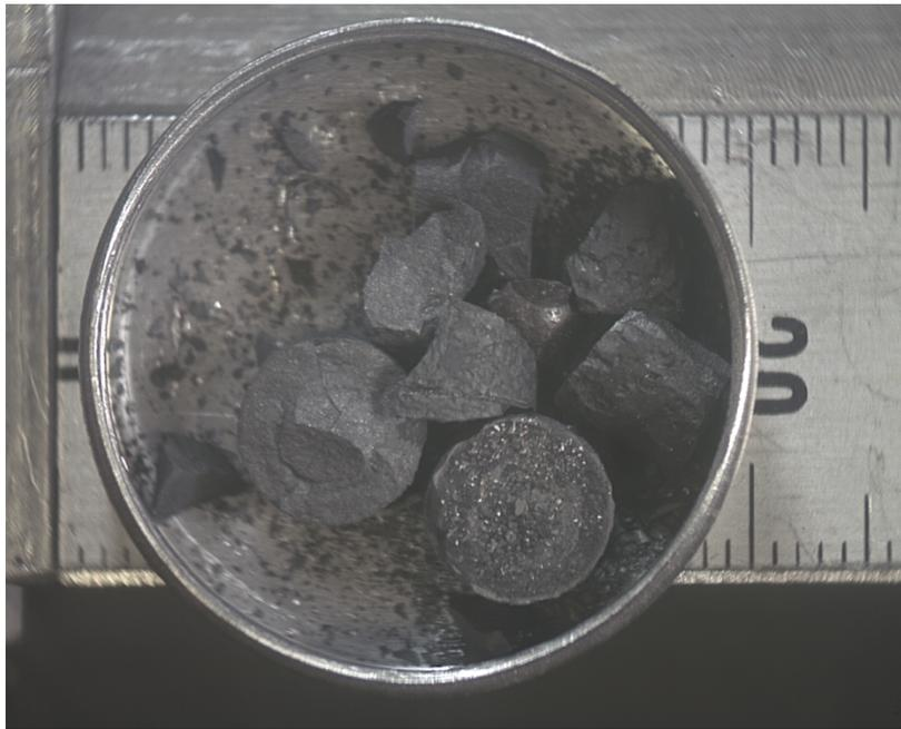
**Figure 2-71 Fuel fragments collected from the bottom of rod 196 after gentle shaking just before gamma scan**
