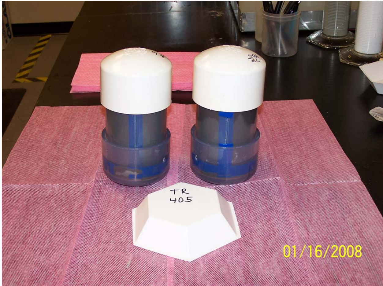
Figure 3-9 Photograph of the molds in which the samples were cast and cured for 28 days prior to removal and measurement at MACTEC (TR 405 is the mix containing MF 816 and slag).
