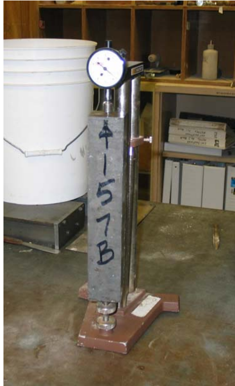
Figure 3-7 Cast bar in a micrometer used to measure shrinkage and expansion (N-Area)
