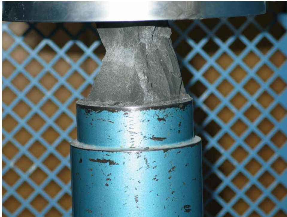
Figure 3-2 One of the cubes immediately after failure of compressive strength testing
