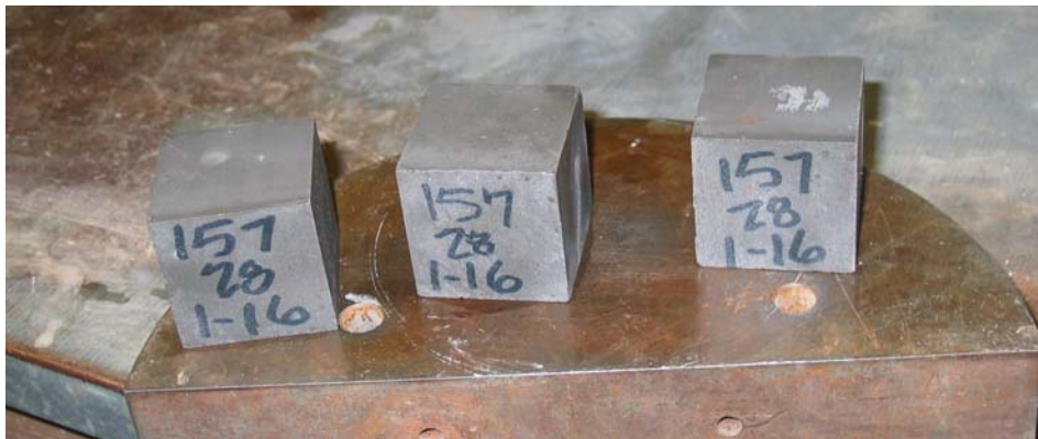
Figure 3-2 The 2 inch cubes immediately after removal from the lime saturated bath and just prior to testing.
