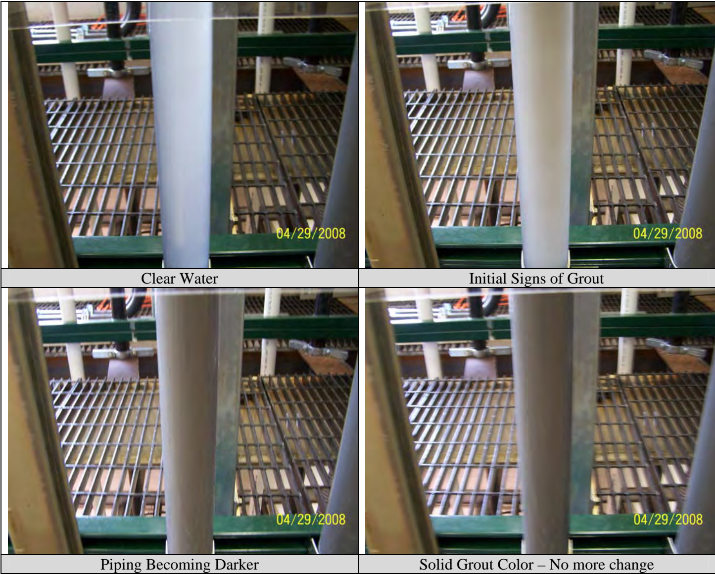
Figure 3-1 Water to Grout Transition in Vertical Cooling Coil Assembly
