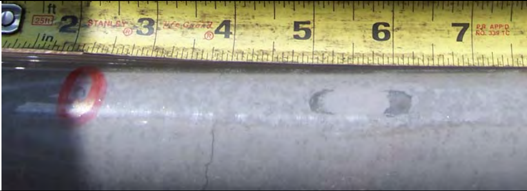
5A – Top View of Pipe, small hole on left, large hole on right
