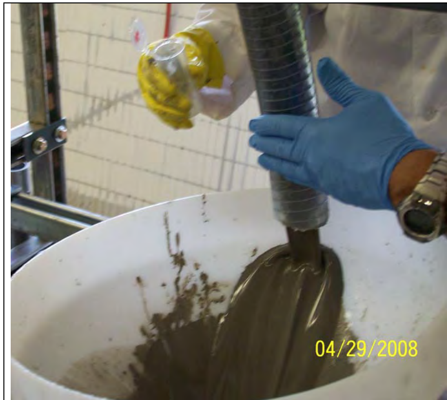
Figure 3-3 Typical Grout Discharging the Vertical Cooling Coil Assembly - Sampling
