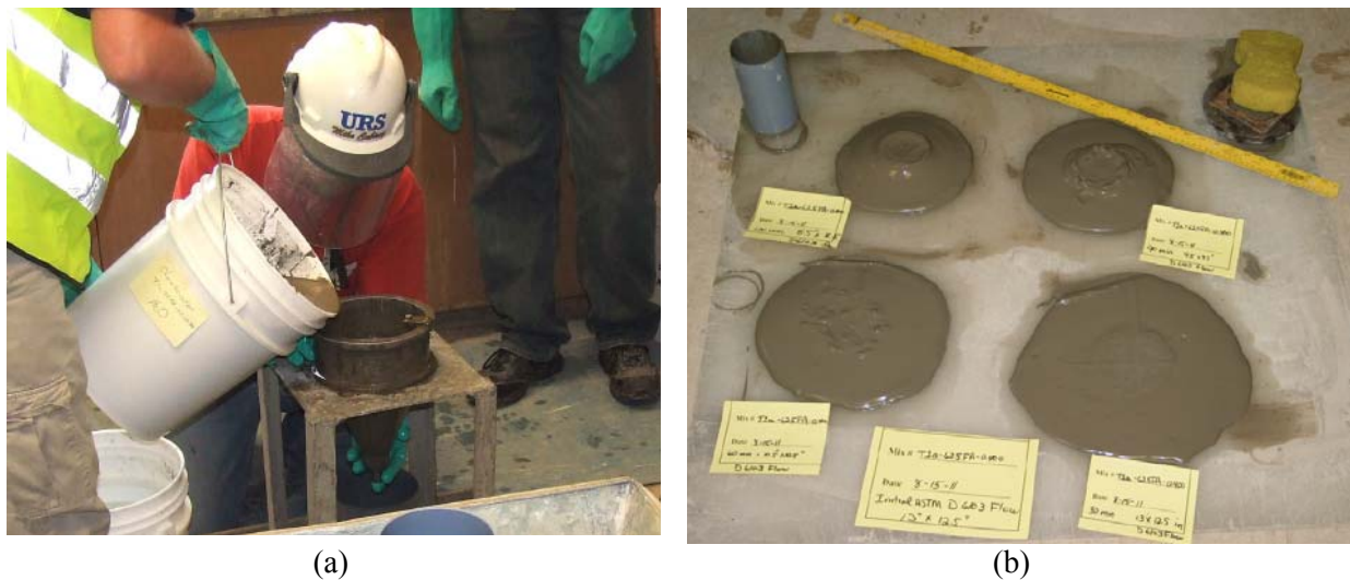
Figure 3-2. Examples of (a) ASTM C939 flow cone measurement and (b) Modified ASTM D6103 flow under initial and static conditions.
