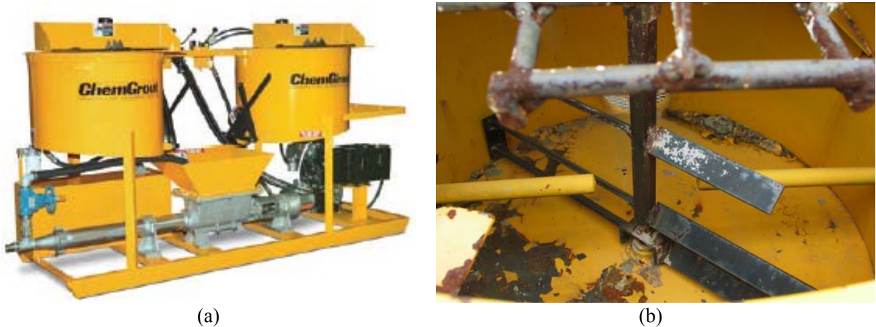
Figure 1-2. (a) ChemGrout™ GC-500-DH skid mounted equipment used in the full-scale cooling coil grout mixing and placement demonstration and (b) view of paddle blades inside mixing tank.
