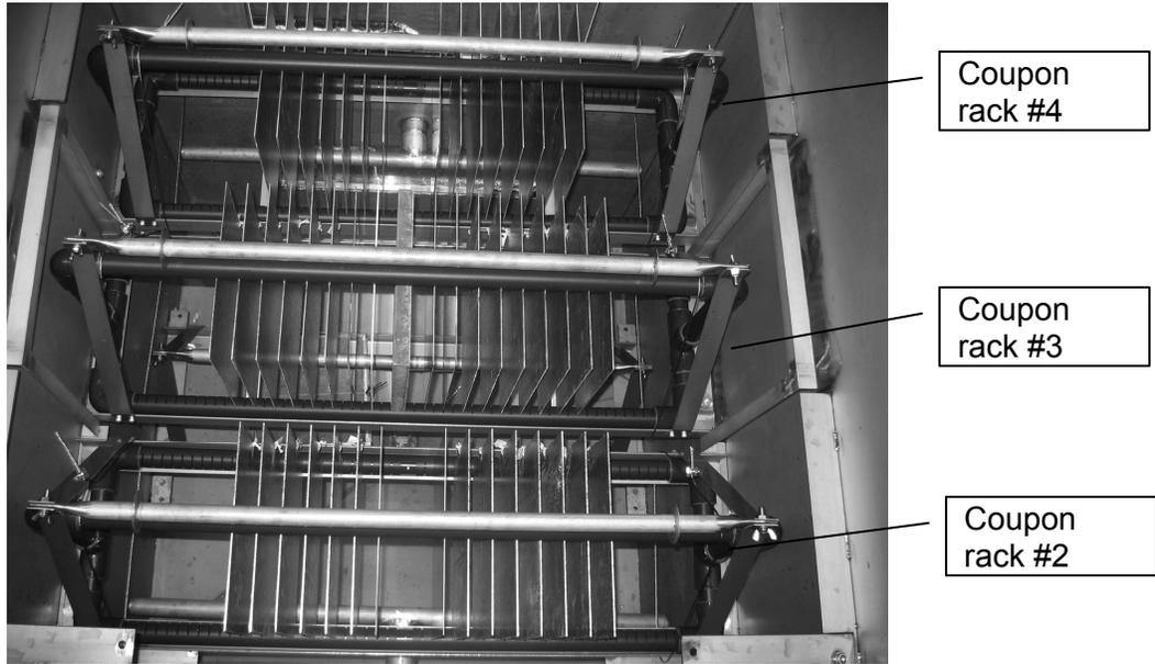
**Figure 4.1-4 Coupon Racks #2,#3,#4 in Test Tank**
