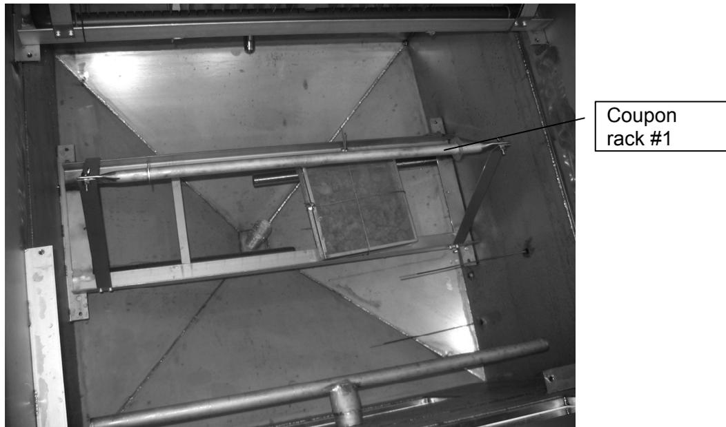
**Figure 4.1-3 The NUKON™ Fiber Glass Holder Made of Stainless Steel Mesh with Sample on Coupon Rack #1**
