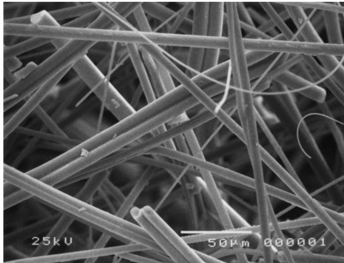
Figure 4.1-8 SEM Image of NUKON™ Fiberglass before Test
