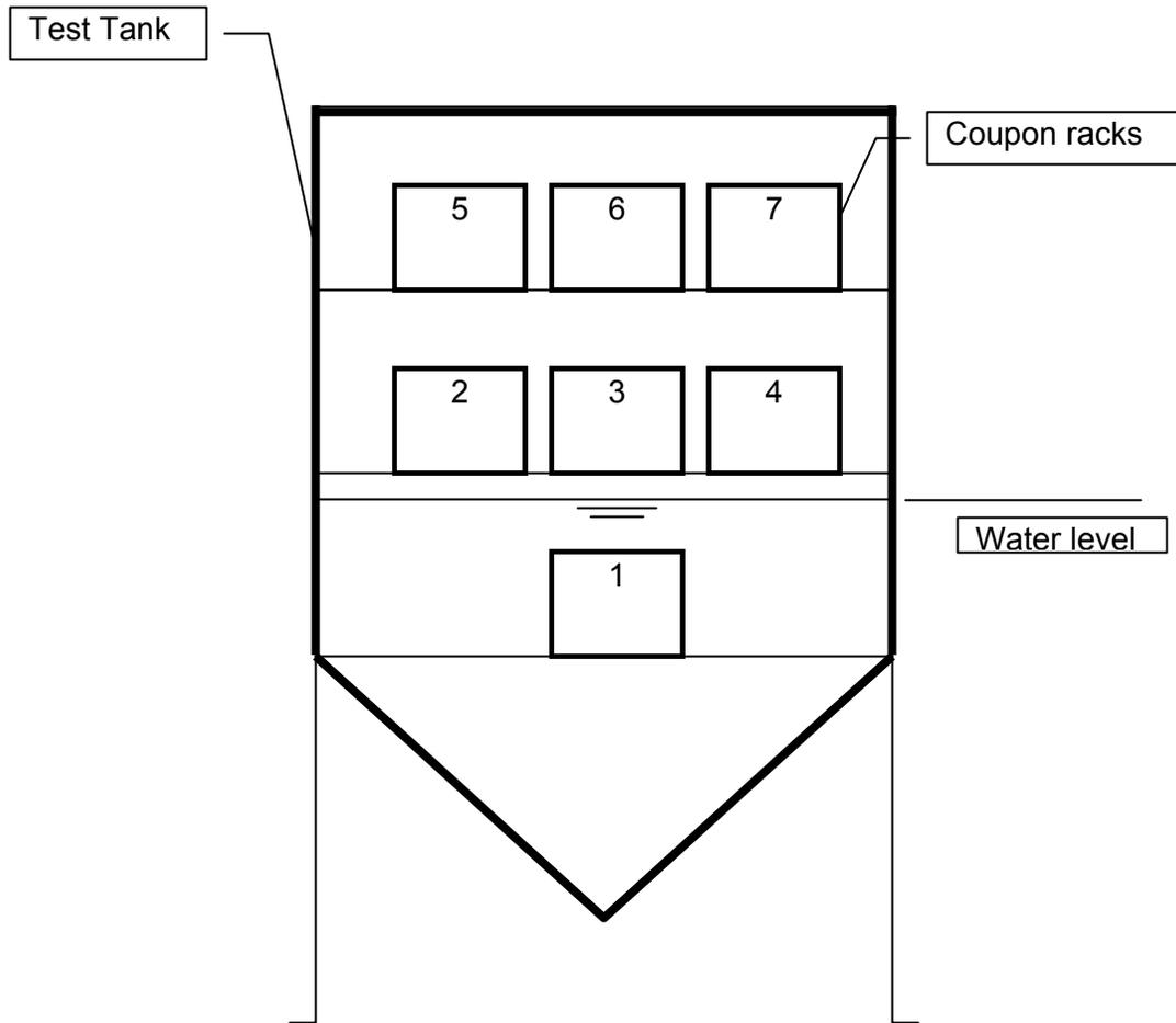
**Figure 4.1-2 The Position of the Coupon Racks in a Test Tank:
