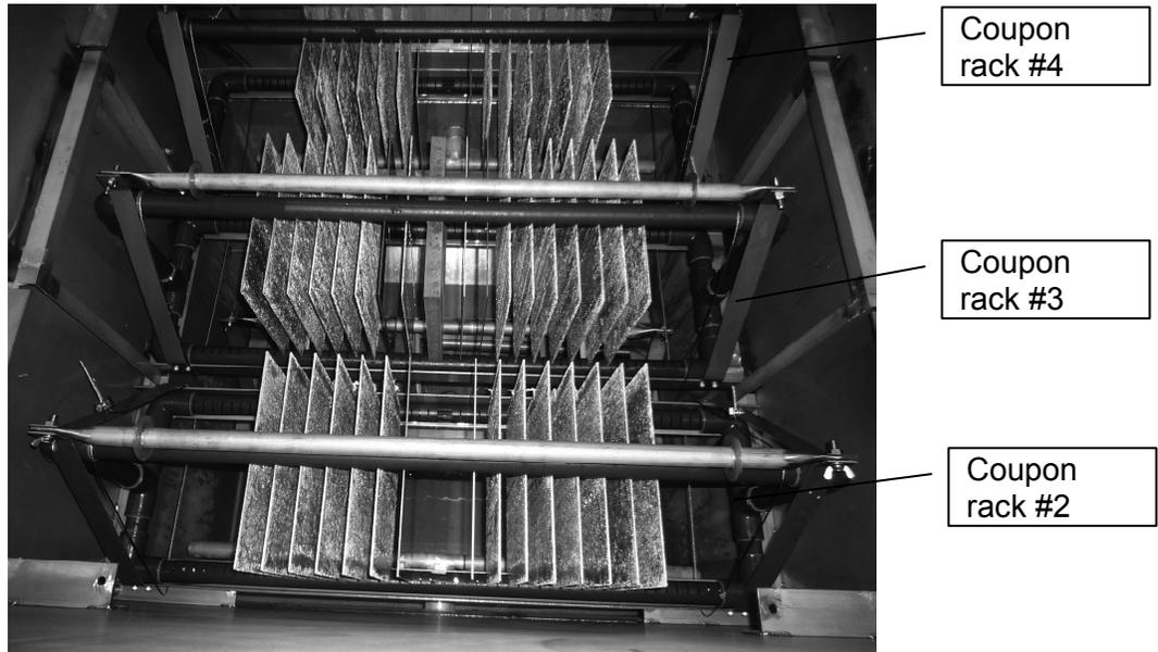
**Figure 4.1-6 Coupon Racks #2,#3,#4 after Test**
