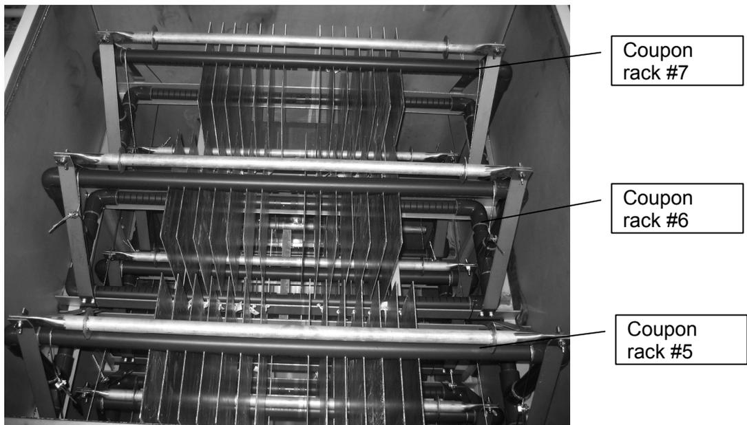
**Figure 4.1-5 Coupon Racks #5,#6,#7 in Test Tank**
