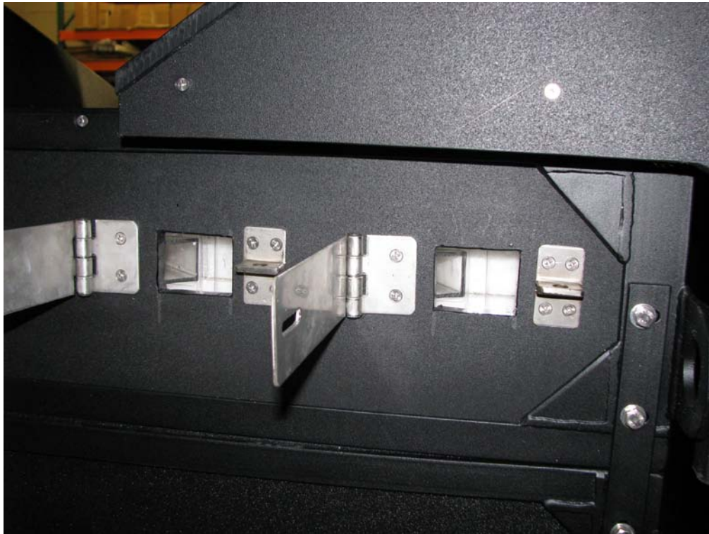
Detail photo of source access for SABIA X-1 analyzer, with locks open, ready for installation of source holders into two source locations. The source access for the SABIA model X1-XP is similar in design, utilizing identical components for the internal guide tube, locking hasps, and source holders.
