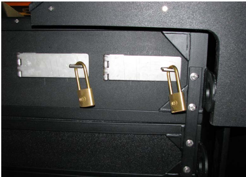
Detail photo of the source housing for the SABIA X-1 analyzer, showing locked source access for two source locations. Not shown in this photo is the Radiation sign, above, and the stainless steel device label, which is placed to the left of the source access locations. The details for the SABIA X1-XP slurry analyzer are similar, with identical locks and locking details.
