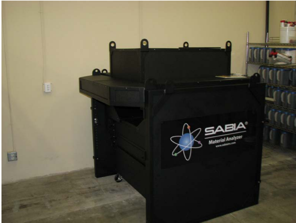
Photo showing a typical SABIA X1 analyzer. This unit is normally mounted on the rails of a conveyor belt. This specific device is used at SABIA for testing of electronics and for testing of materials.
