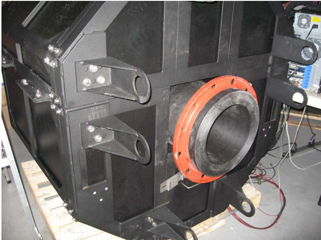
Partial view of the top of the SABIA X1-XP analyzer, showing the hasp of the source access below the pipe. This unit was designed for operation in a vertical orientation with a 12 inch pipe (installed)
