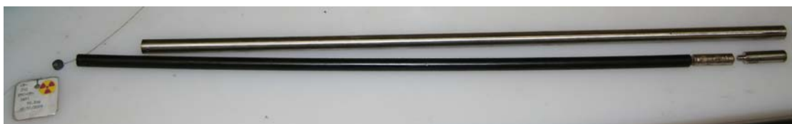
Internal components of source holder, showing stainless steel source holder housing, source ID tag, polyethylene rod (moderator and shielding for neutrons), bismuth (shield for source gamma radiation), and source. Assembly is performed by SABIA, including inserting source into stainless steel source holder housing, followed by bismuth shield, polyethylene rod, and then wire seal and source ID tag. Engineering drawing of the source holder is shown on SABIA drawing 1002993, Revision C.
