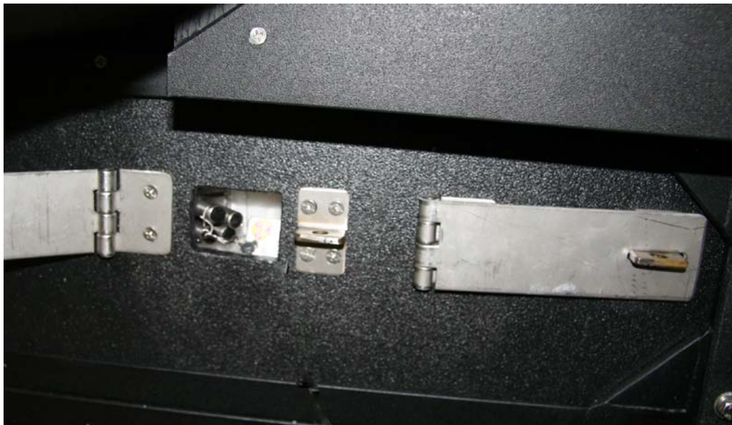
Detail photo of source housing of SABIA X-1 analyzer, showing source holders installed into one source location.
