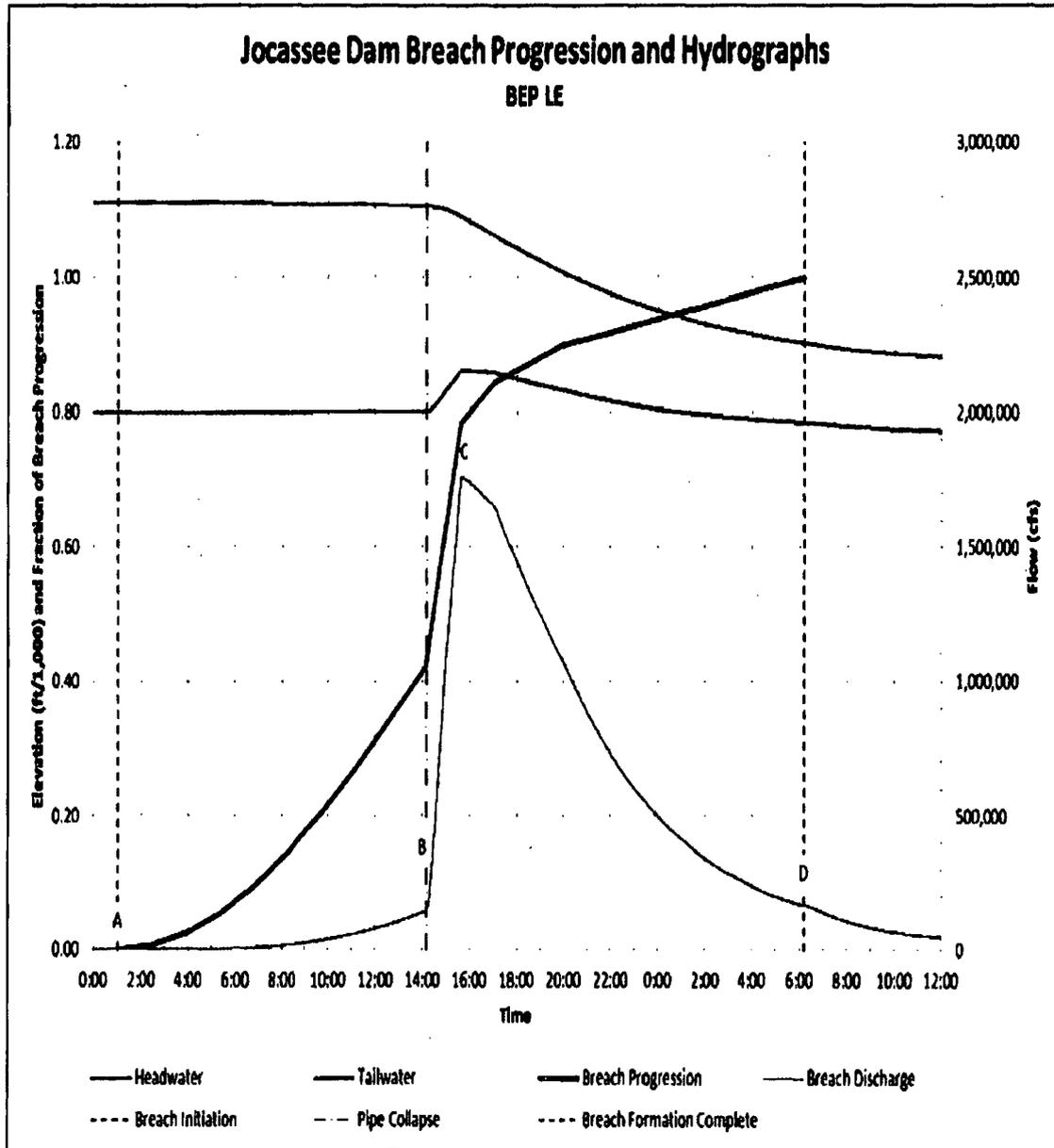
**Breach Formation Time:** Xu & Zhang definition: - 29.2 (13.2 hours piping + 16.0 hours open weir) Froehlich definition: -16.0 hours open weir
