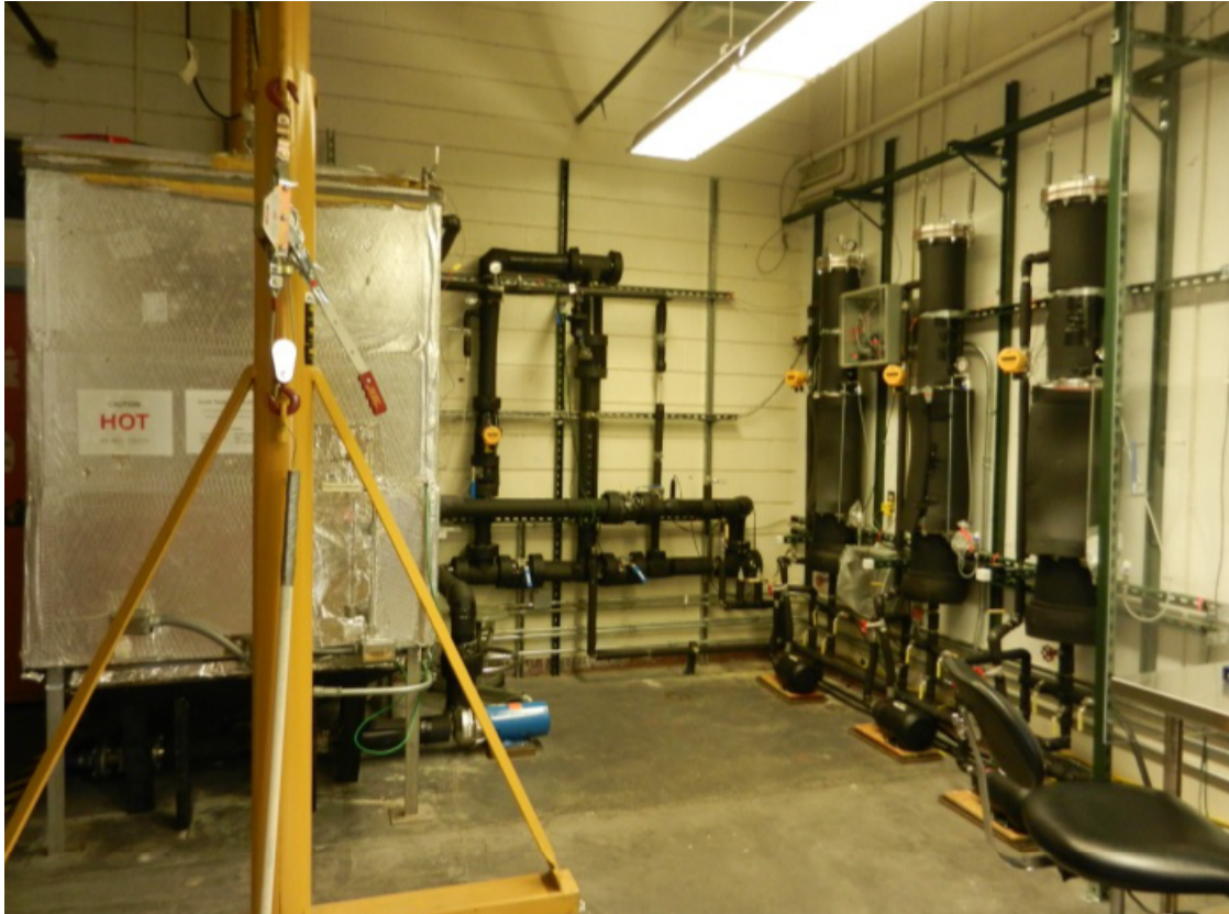
Figure 1. Chemical Effects Head Loss Tank (left) and head loss columns (right).
