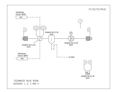
kte – nuclear Island Drain and vent systems – Floor Drains 3 onx – operational chilled water system sam3 – main steam and main feedwater valve room ventilation system
