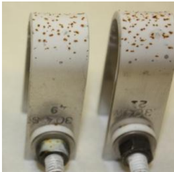
Specimens with 10 g/m 2 Salt, Exposed to Cyclic Humidity (15 to 30 g/m 3 ) at 45 °C for 4 Months
