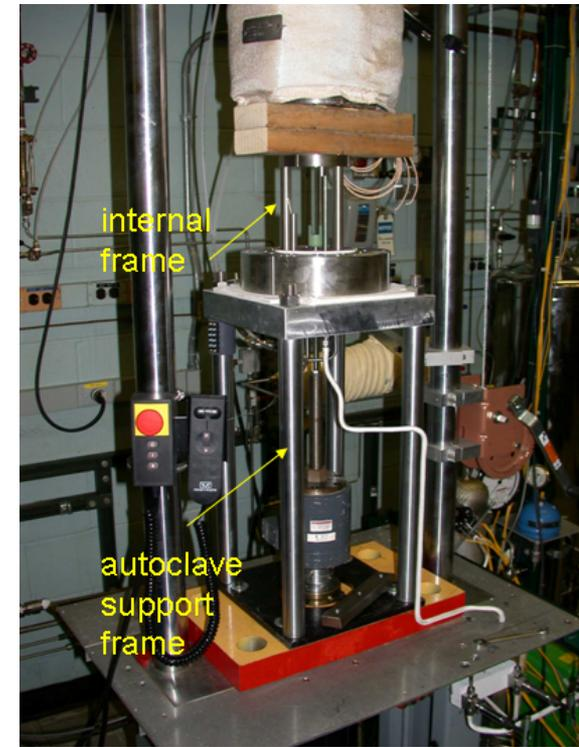
Crack growth rate test systems located at ANL used to obtain accurate crack growth rates
