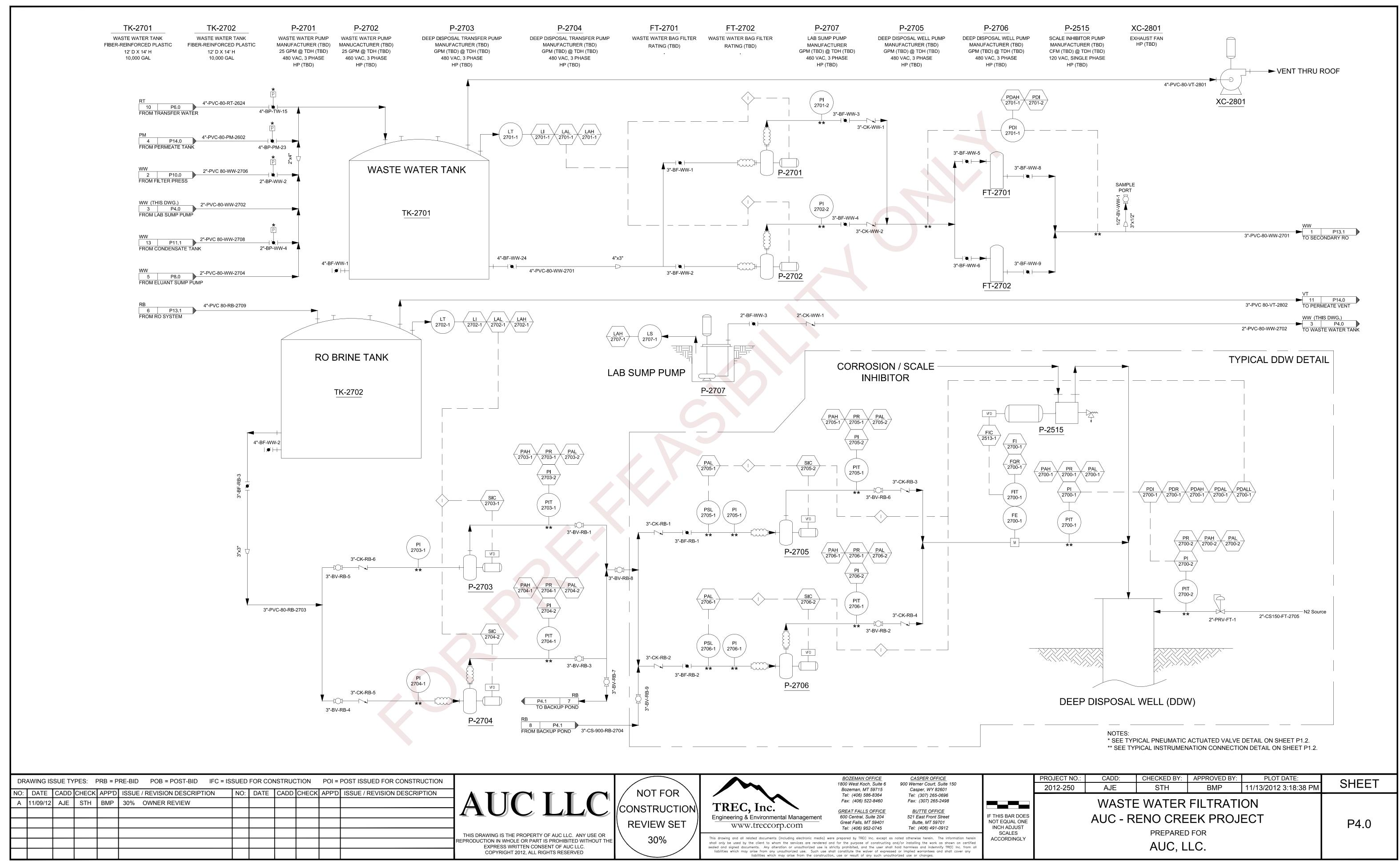
PD-2701 P-2713 BACKUP POND VOLUME (TBD) BACKUP POND PUMP MANUFACTURER (TBD) GPM (TBD) @ TDH (TBD) 480 VAC, 3 PHASE HP (TBD) FLOW SLEEVE RB
