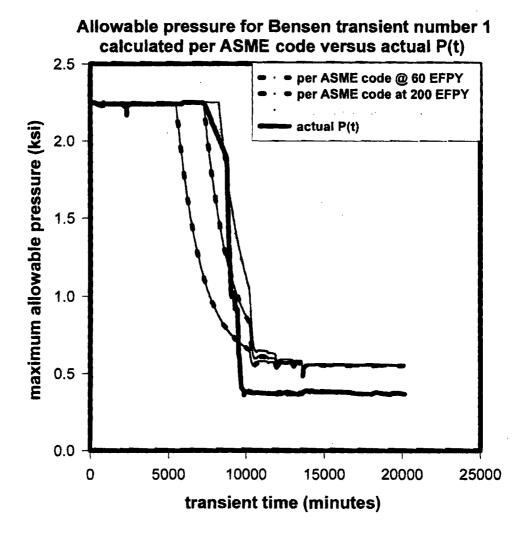
Figure 1 – using h = 10000: actual P(t) transgresses the maximum allowable pressure curve derived per ASME code for 60 and 200 EFPY, but appears to **nearly** comply with the maximum allowable pressure curve derive by the ASME method at 32 EFPY.
