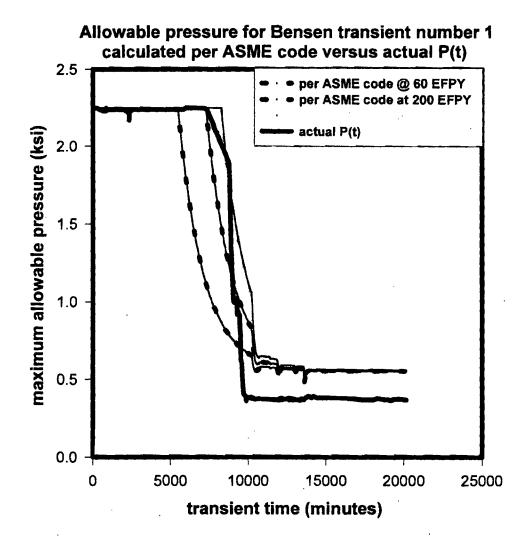
Figure 1 – using h = 10000: actual P(t) transgresses the maximum allowable pressure curve derived per ASME code for 60 and 200 EFPY, but appears to **nearly** comply with the maximum allowable pressure curve derive by the ASME method at 32 EFPY.
