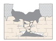
The cavity eventually breaches the ground surface, creating sudden and dramatic sinkholes.
