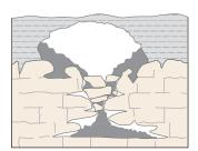
The cavity migrates upward by progressive roof collapse.
