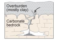
Sediments ravel into a cavity.
