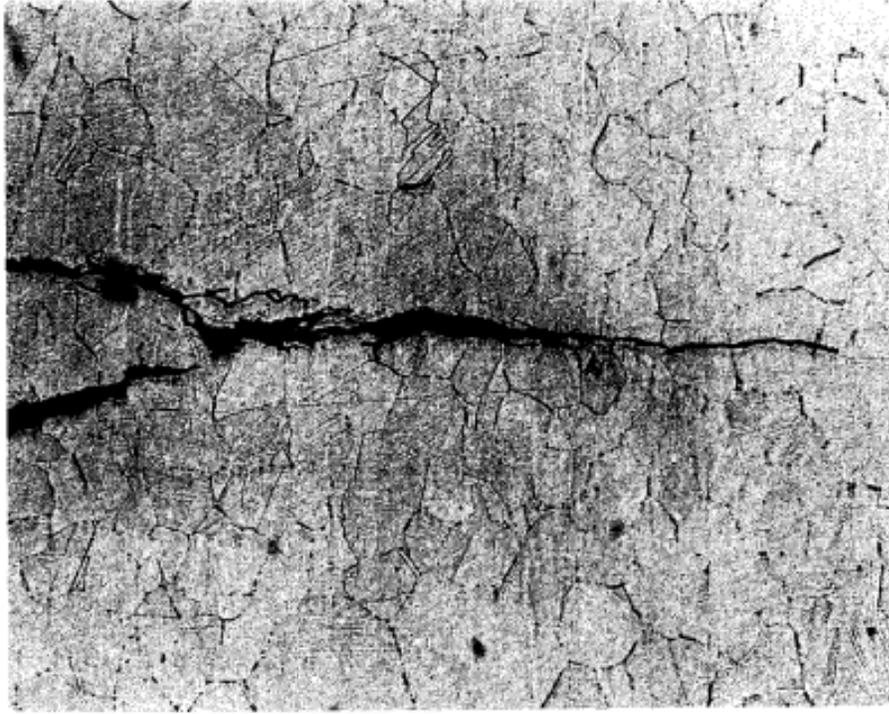
**Type 304 stainless steel piping contaminated with chlorides. Crack depth is about 1.2 mm(50 mils) (Stein, et al., 1986). (permission from ASM International)**
