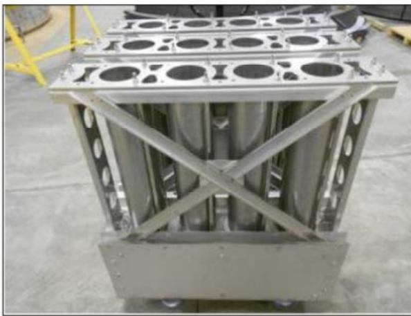
Figure 3-2: Strainer Prototype
