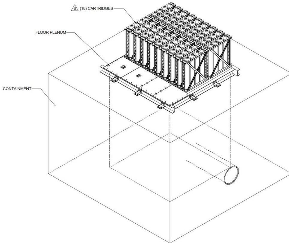
Figure 3-1: Plant Recirculation Sump Strainer
