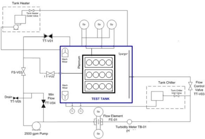
Figure 4-1: Example Tank Piping and Instrumentation Diagram
