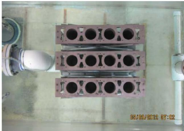
Figure 3-3: Strainer Prototype in Tank, Top View
