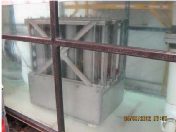
Figure 3-4: Strainer Prototype in Tank
