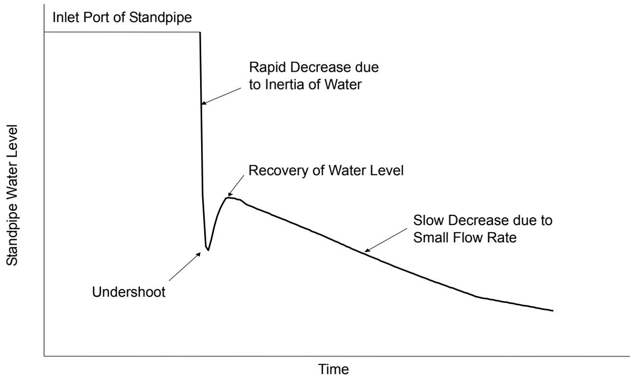
**Fig.2.2.1-3 Example of Water Level Transient in Standpipe (Schematic Chart)**
