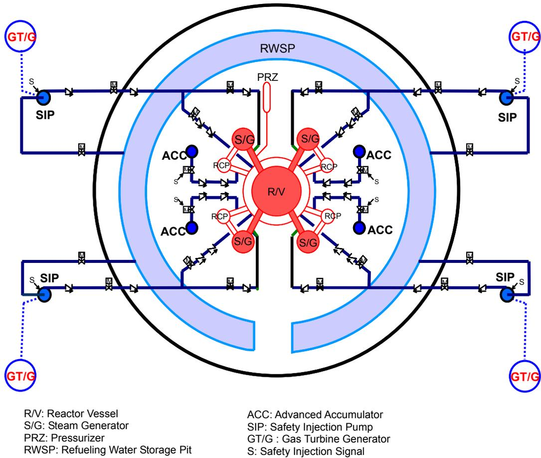
Fig. 2.1-2 System Configuration of the US-APWR ECCS
