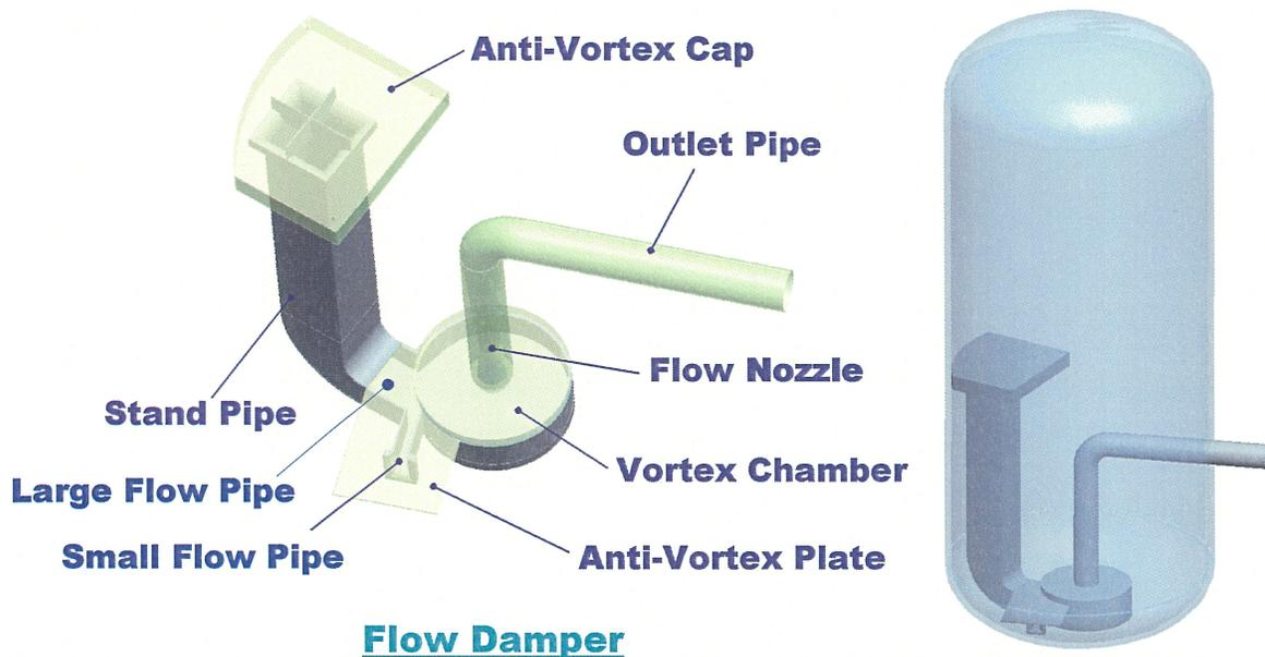
Fig. 3.3-1 Overview of the Flow Damper
