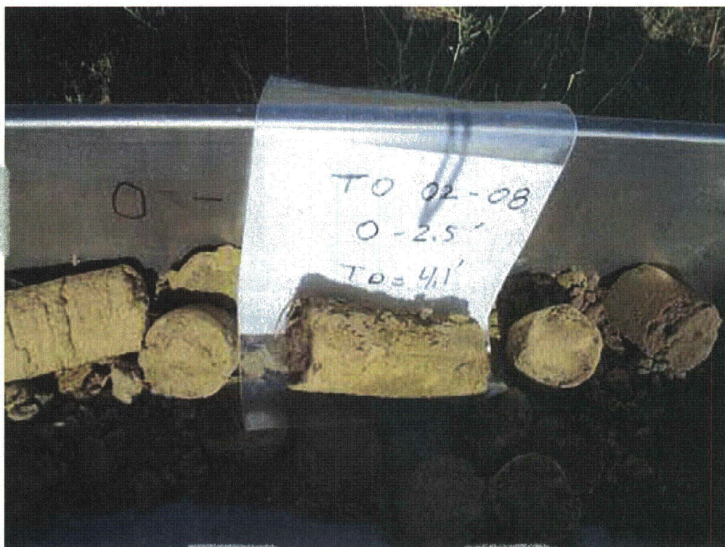
Figure 28. Soil Samples Collected Using the Geoprobe
