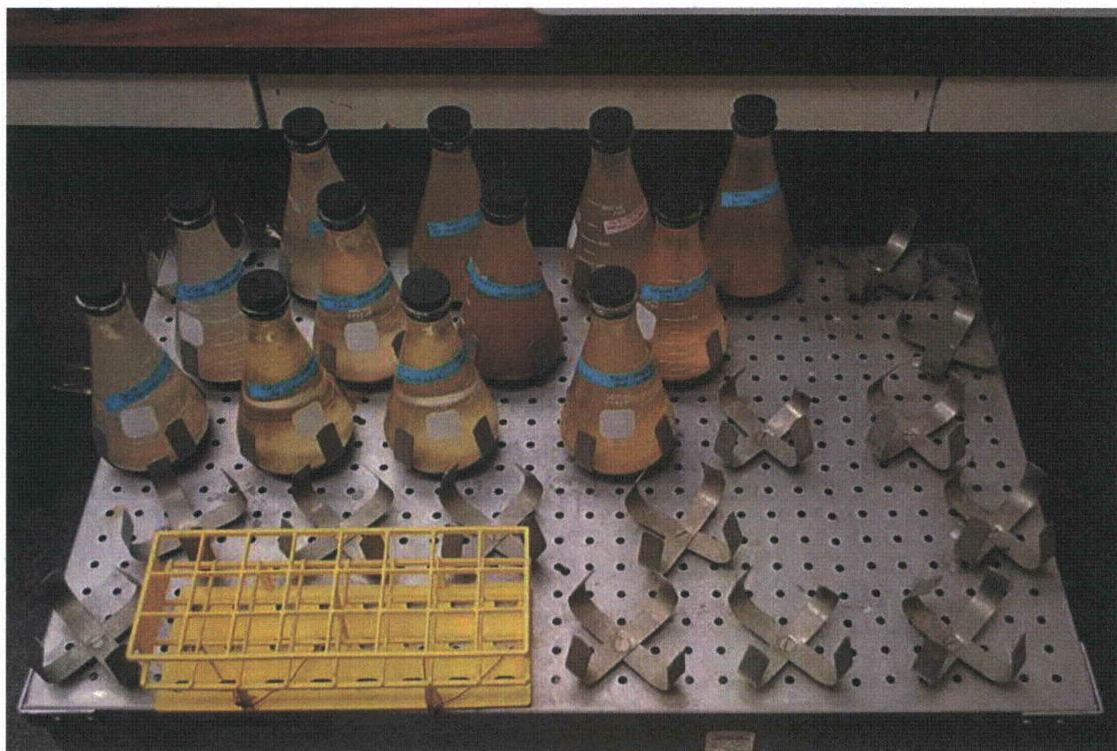
Figure 5. CARB Extractions on Orbital Shaker Table
