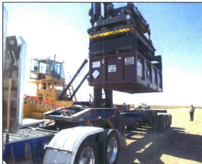
Figure 2. Photo of Taylor industrial forklift placing a loaded IMC onto a BED truck.
