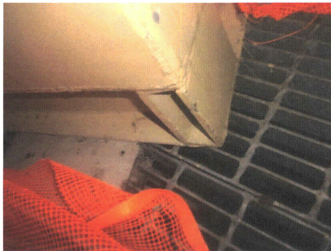
Missing welds from 23 Iodine Removal Unit base
