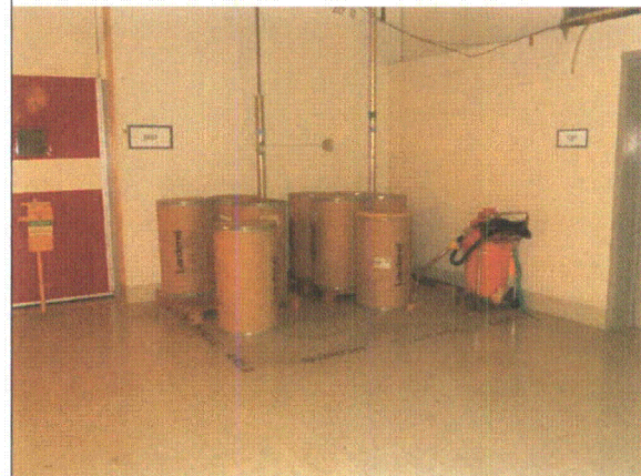
Note: Pallets, drums and vacuum not secured.
