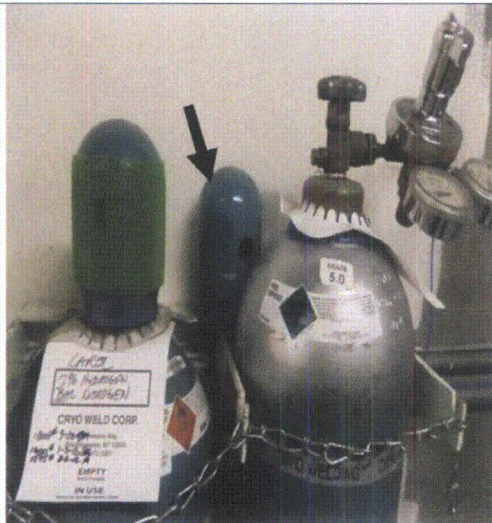
Note: Loose cap behind the compressed air bottles.
