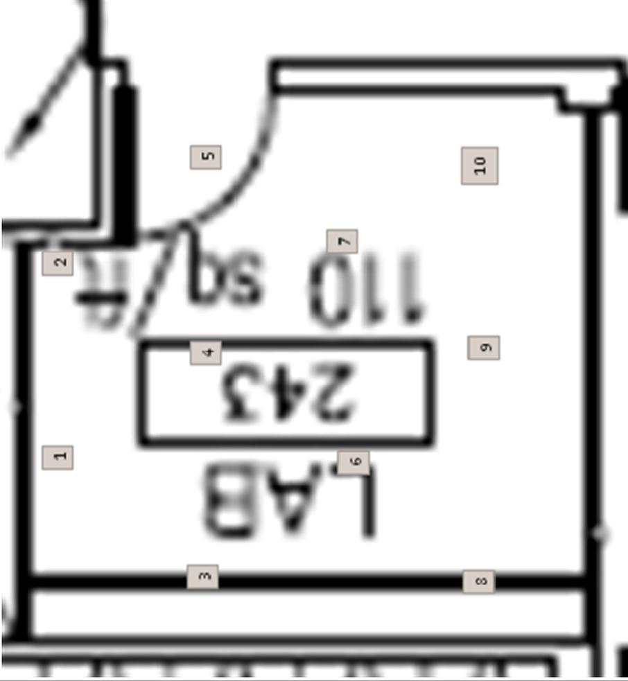
**REMARKS: Systematic Floor Survey** Random Start Point was determined by random sample generator. Location 4 is the random start at 4ft west and 3ft south. The NW corner was the 0/0 location. The grid was marked out on a 3ft N-S separation and a 4ft E-W separation to acquire a triangular grid pattern.
