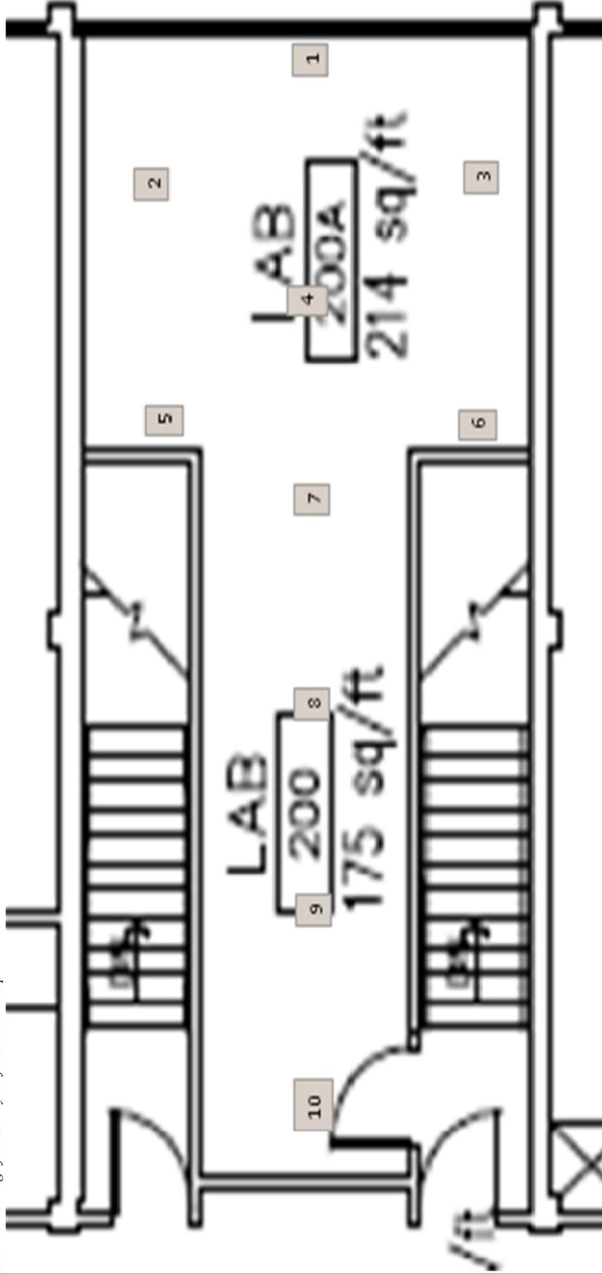
REMARKS: **Systematic Floor Survey** Random Start Point was determined by random sample generator. Location 9 is the random start at 7ft west and 25ft south. The NW corner was the 0/0 location. The grid was marked out on a 6ft N-S separation and a 5ft E-W separation to acquire a triangular grid pattern.
