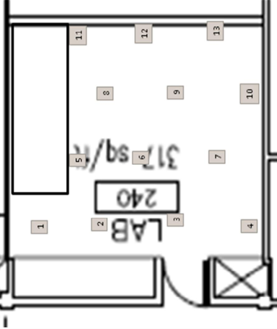
REMARKS: **Systematic Floor Survey** Random Start Point was determined by random sample generator. Location 3 is the random start at 3ft west and 12ft south. The NW corner was the 0/0 location. The grid was marked out on a 4ft N-S separation and a 3ft E-W separation to acquire a triangular grid pattern.
