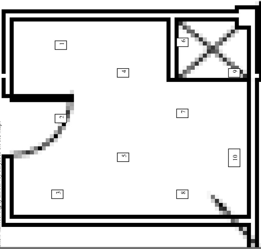
**REMARKS:** Systematic Floor Survey Random Start Point was determined by random sample generator. Location 8 is the random start at 7ft east and 3ft south. The NW corner was the 0/0 location. The grid was marked using a triangular grid pattern.
