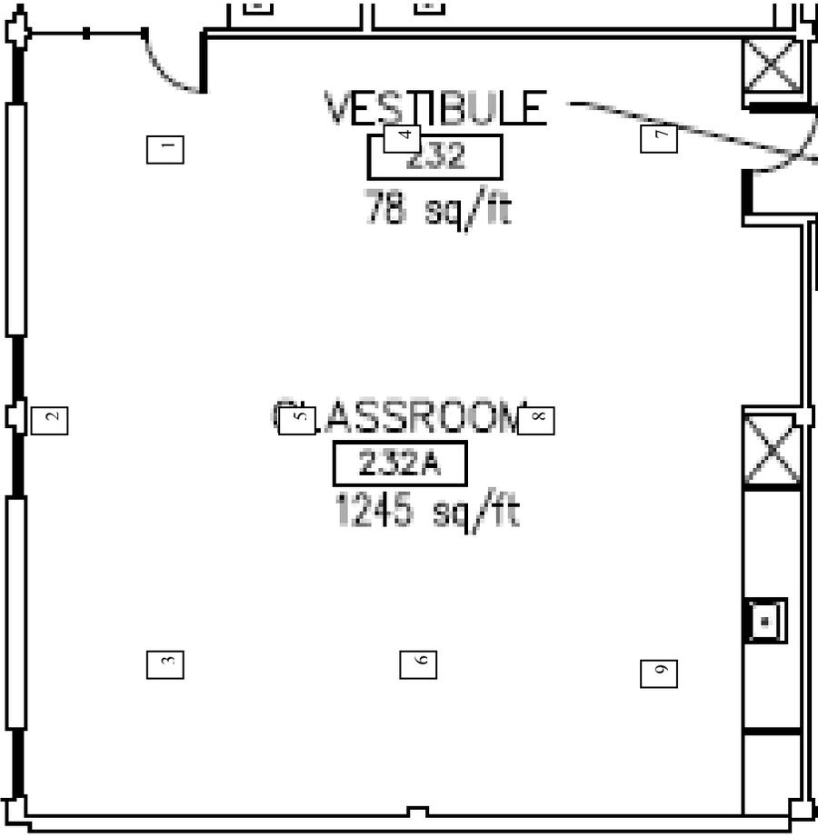
REMARKS: Systematic Floor Survey Random Start Point was determined by random sample generator. Location 8 is the random start at 22ft east and 15ft south. The NW corner was the 0/0 location. The grid was marked using a triangular grid pattern.
