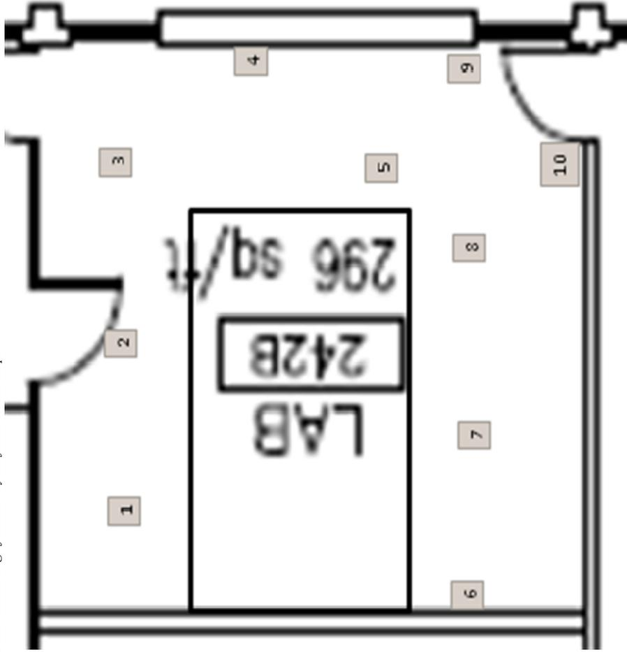
REMARKS: **Systematic Floor Survey** Random Start Point was determined by random sample generator. Location 3 is the random start at 12ft west and 3ft south. The NW corner was the 0/0 location. The grid was marked out on a 3ft N-S separation and a 4ft E-W separation to acquire a triangular grid pattern.
