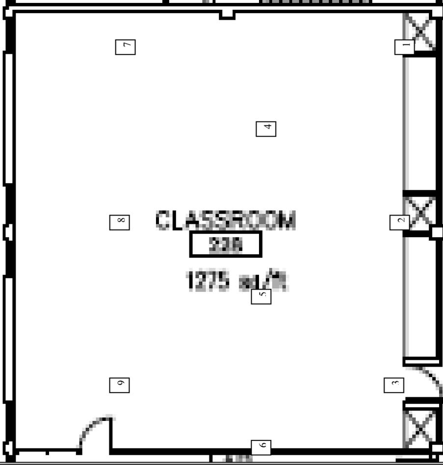
REMARKS: Systematic Floor Survey Random Start Point was determined by random sample generator. Location 5 is the random start at 22ft east and 12ft south. The NW corner was the 0/0 location. The grid was marked using a triangular grid pattern.
