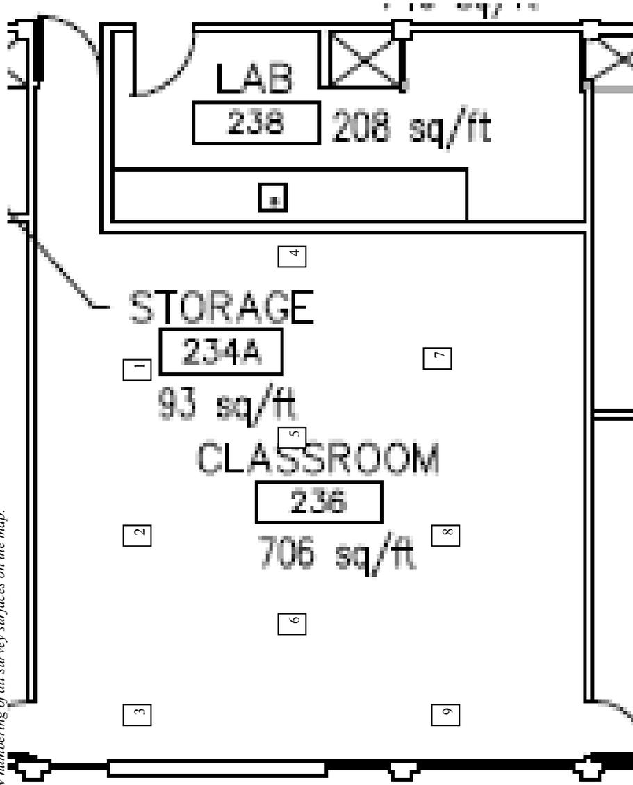
REMARKS: **Systematic Floor Survey** Random Start Point was determined by random sample generator. Location 5 is the random start at 8ft east and 20ft south. The NW corner was the 0/0 location. The grid was marked using a triangular grid pattern.
