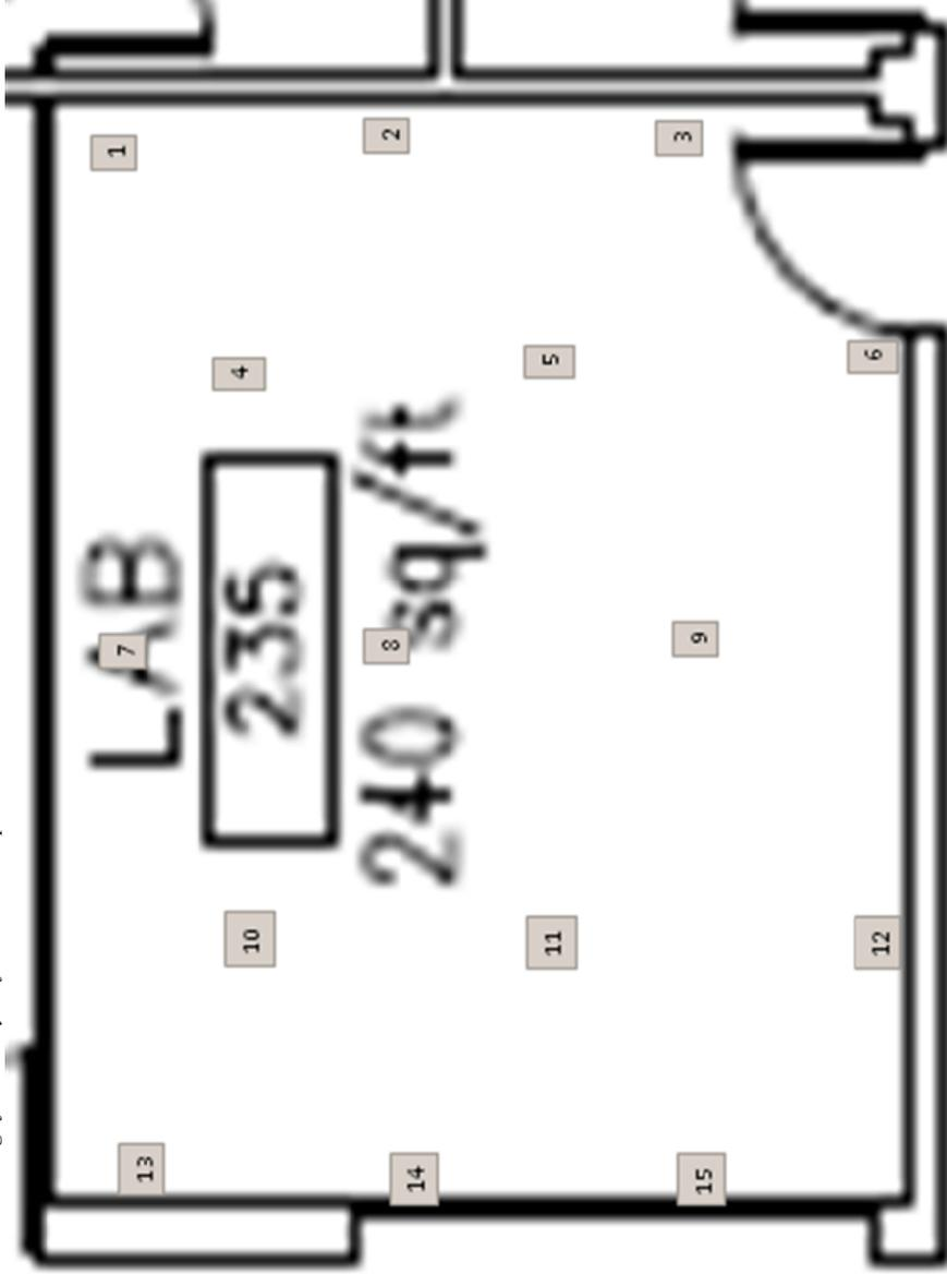
**REMARKS:** Systematic Floor Survey Random Start Point was determined by random sample generator. Location 13 is the random start at 11ft west and 17ft south. The NW corner was the 0/0 location. The grid was marked out on a 4ft N-S separation and a 5ft E-W separation to acquire a triangular grid pattern.
