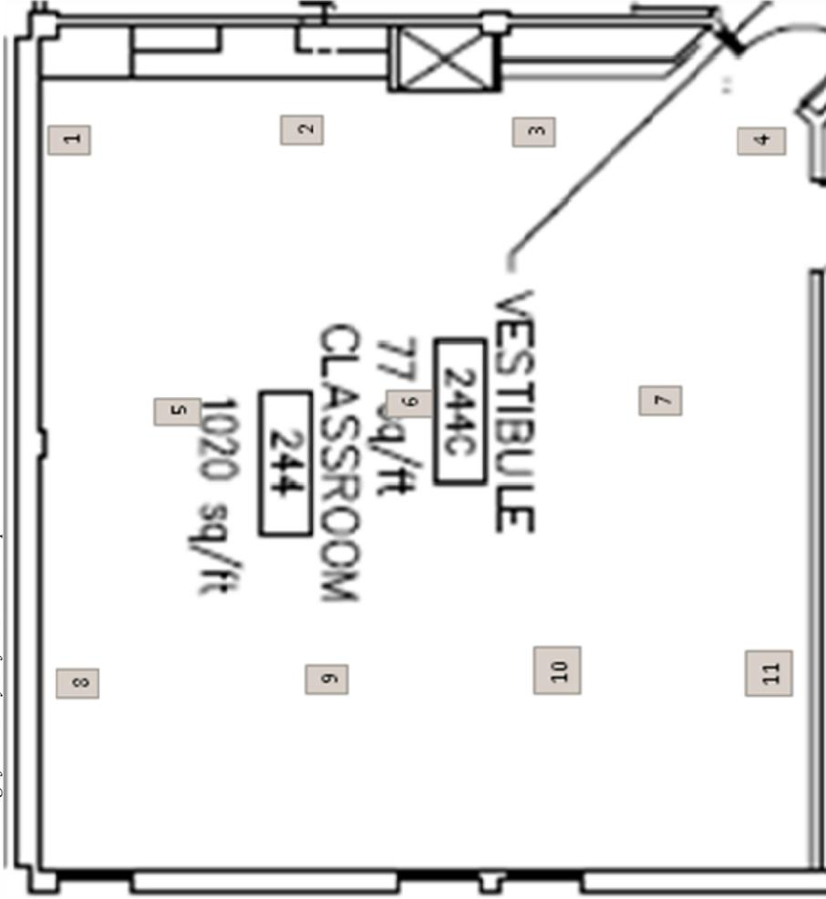
REMARKS: **Systematic Floor Survey** Random Start Point was determined by random sample generator. Location 8 is the random start at 4ft west and 24ft south. The NW corner was the 0/0 location. The grid was marked out on a 9ft N-S separation and a 8ft E-W separation to acquire a triangular grid pattern.
