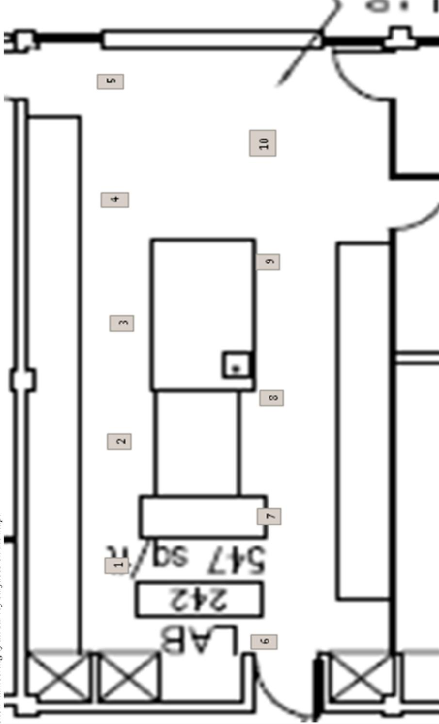
REMARKS: **Systematic Floor Survey** Random Start Point was determined by random sample generator. Location 2 is the random start at 11ft west and 6ft south. The NW corner was the 0/0 location. The grid was marked out on a 5ft N-S separation and a 6ft E-W separation to acquire a triangular grid pattern.
