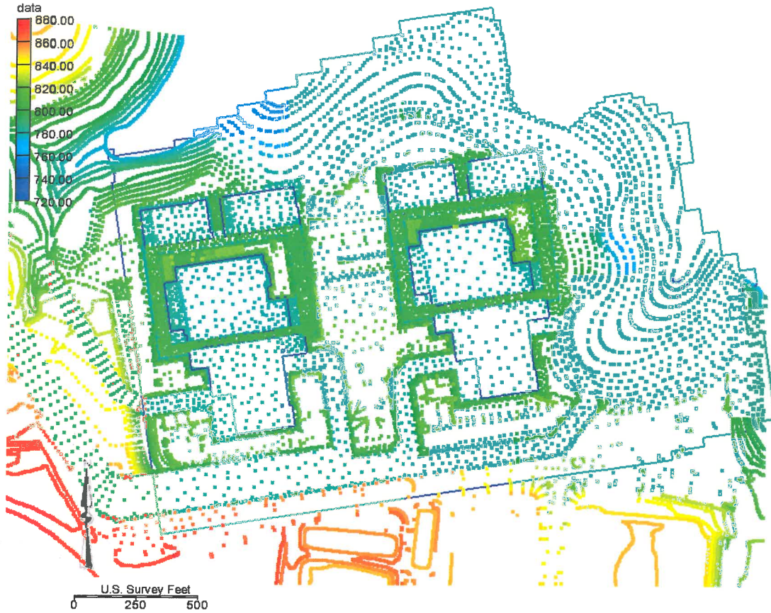
Figure 5-5. Elevations of Composite Top of Bedrock Surface Across the Model Domain.
