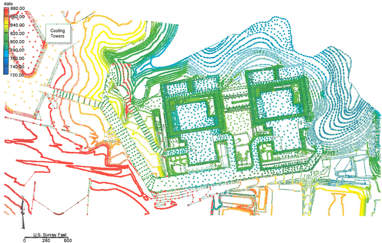
Figure 5-9. Planned Top of Bedrock Surface Across Site, Color Indicates Elevation as Shown in Legend (ft msl).
