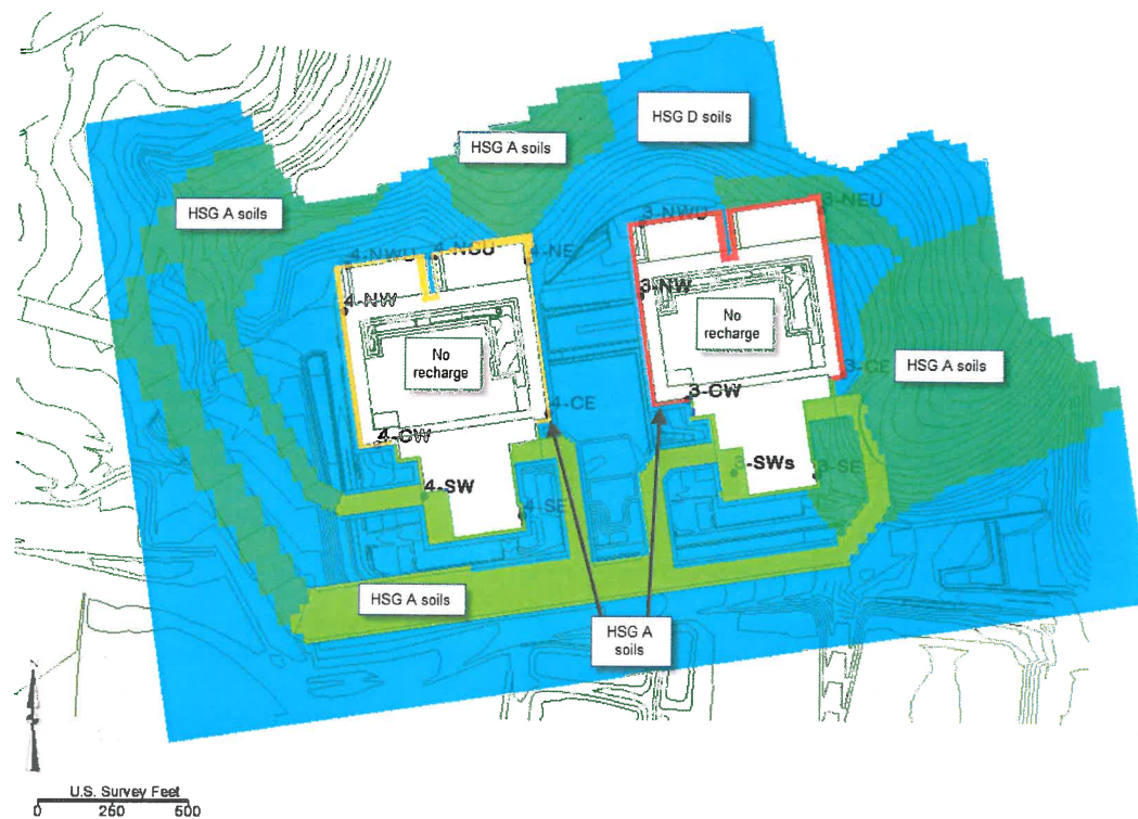
Figure 5-15. Recharge Zones Across the MODFLOW Model Domain
