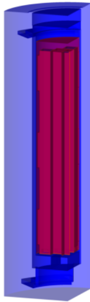
Figure-2.2 Sectional View of VSC-17 Dry Storage System Used in Computation
