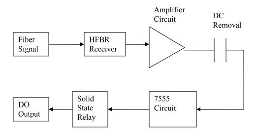
Figure 1: HFC-ILR06 Solid State DO Flow Diagram
