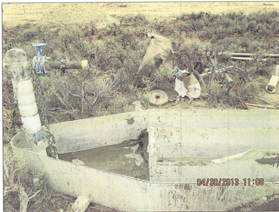
Photo Number 18: This is a view inside the portable mud-pit. It has partitions that route drilling mud through a labyrinth that allows mud to precipitate. The mud that accumulates in the portable mud-pit is transferred into a secondary tank (depicted on the right in Photo Number 17 above).
