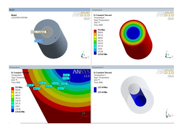
Figure 3.5.6-2 Results of ANSYS Analysis of Payload Vessel Contents Region
