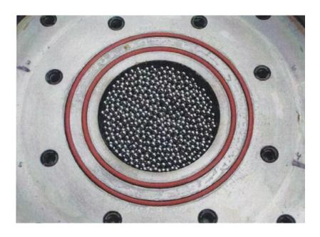
Figure 3.5.6-1 CI-1 Inner Vessel and Gasket Post Fire Test
