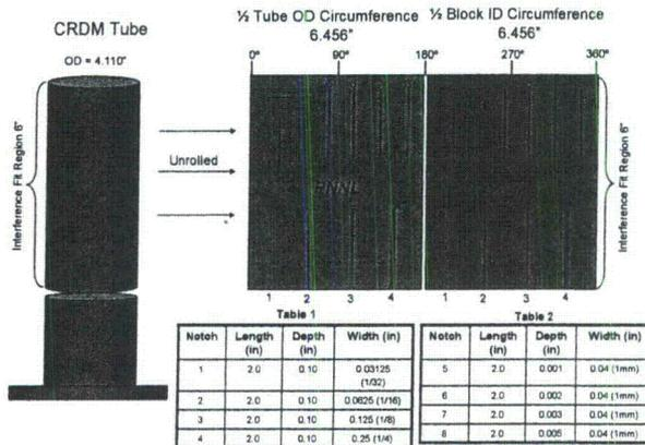
Figure 3. Interference fit #2; notch and pattern design
