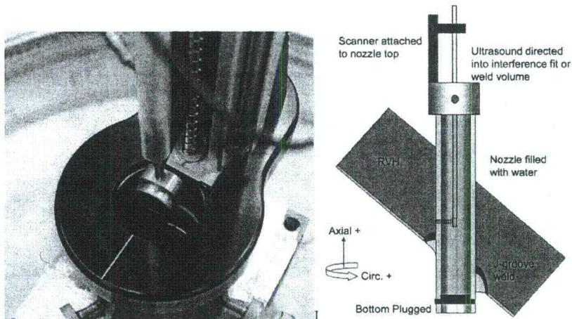
Figure 4. Left: Scanner on Calibration Specimen. Right: Inspection Schematic
