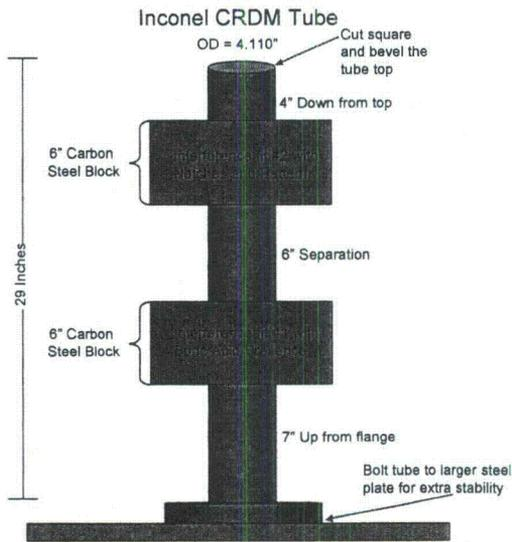
Figure 1. Assembled CRDM interference fit mock-up specimen
