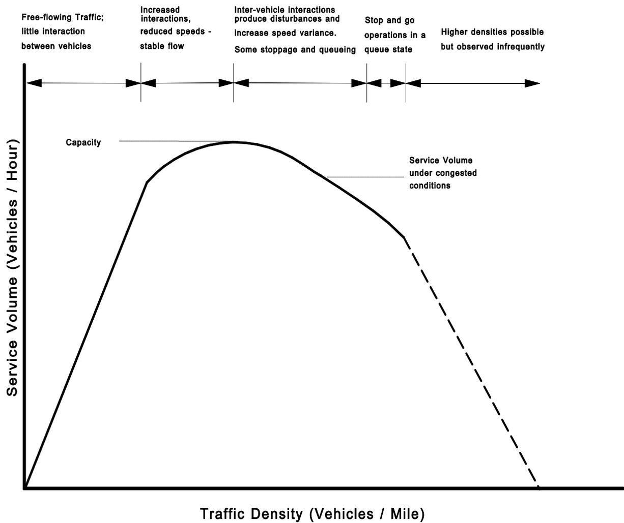
**Figure 4-1. Fundamental Relationship Between Volume and Density**
