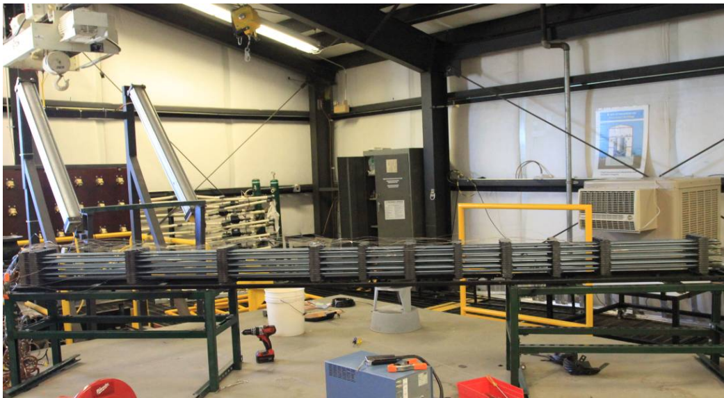
Figure 1. Single fuel assembly for Phase 1 testing in construction stage.
