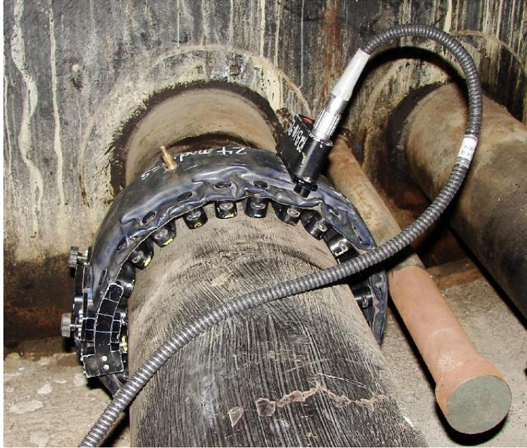
**Figure 4.12.** Application of a Comb Transducer to the Inspection of a Pipe (EPRI 2008). Reproduced with permission from Electric Power Research Institute, Palo Alto, California.
