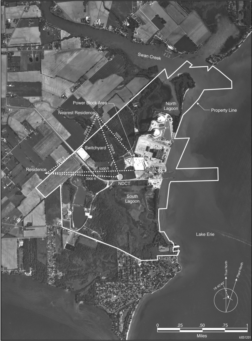
Figure 4-7. Major Noise Sources and Nearby Sensitive Receptors during Building of Fermi 3
